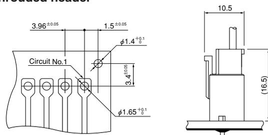
Note: 1. The above figure is the figure viewed from soldering side.
