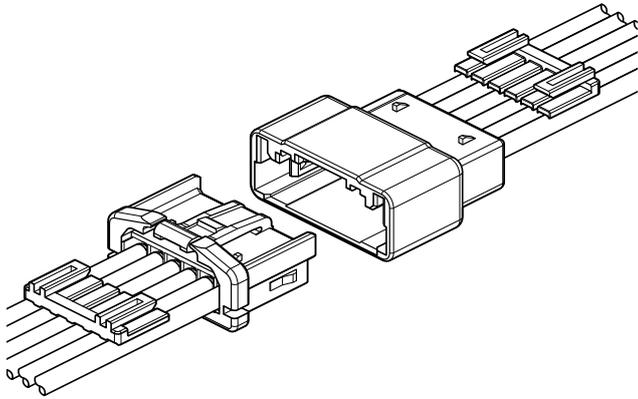
This connector is a 2.5 mm pitch wire-to-wire connector, having incomplete mating prevention mechanism. 2-circuit and 3-circuit connectors have control key to prevent connector from mating with incorrect circuits, thus, several same circuit connectors can be used.
