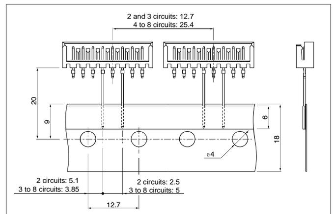
Note: Conforms to JIC C 0806 of "Tape packaging of components with unidirectional leads on continuous tapes".
