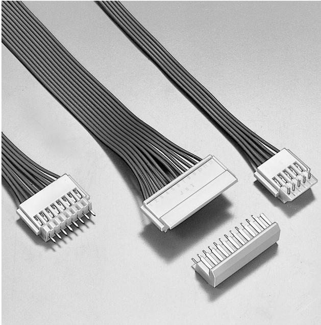
**This 2.5mm pitch connector is used to connect wires to printed circuit boards. The header is available in three configurations: top, side, and bottom entry. This allows the wires to be perpendicular or parallel to the printed circuit board in any direction.**
