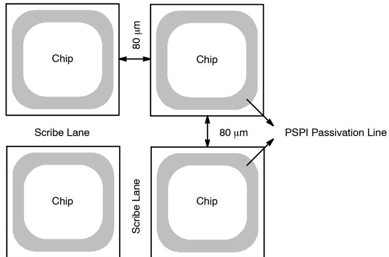
**Figure 3. Saw-on-film Frame Packing Based on Tested Wafer**
