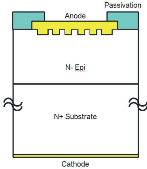
**Figure 2. Cross Section**
