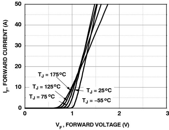
Figure 4. Forward Characteristics
