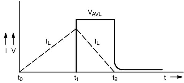
Figure 12. Unclamped Inductive Switching Test Circuit & Waveform
