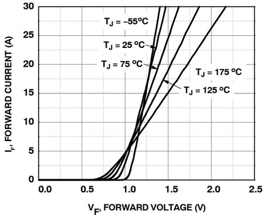
Figure 4. Forward Characteristics
