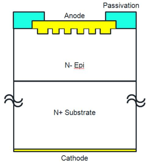
Figure 2. Cross Section
