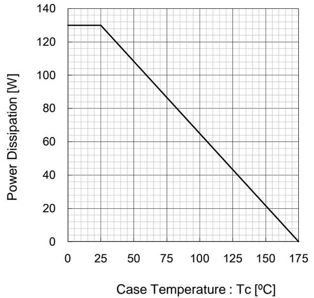
Fig.7 Derating Curve  $I_p$ - $T_c$  (Per leg)
