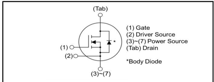
Please note Driver Source and Power Source are not exchangeable. Their exchange might lead to malfunction.
