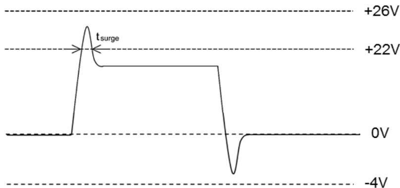
Please note especially when using driver source that  $V_{GSS\_surge}$  must be in the range of absolute maximum rating.
