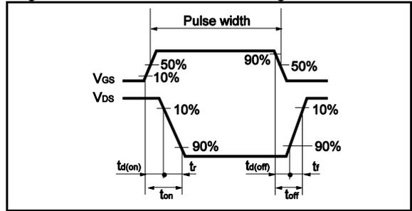
Fig.2-3 Waveforms for Switching Energy Loss
