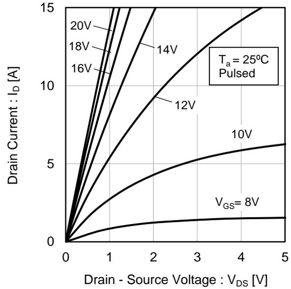
Fig.6  $T_j = 25^\circ C$  3rd Quadrant Characteristics
