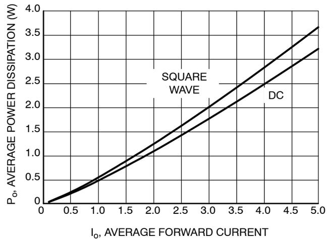
Figure 6. Power Dissipation
