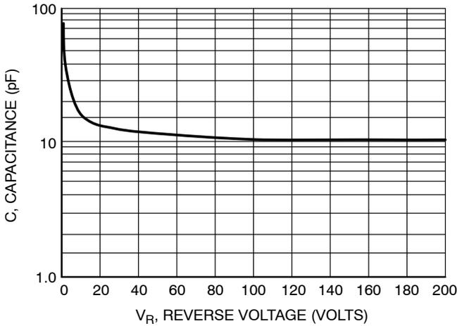
Figure 5. Typical Capacitance
