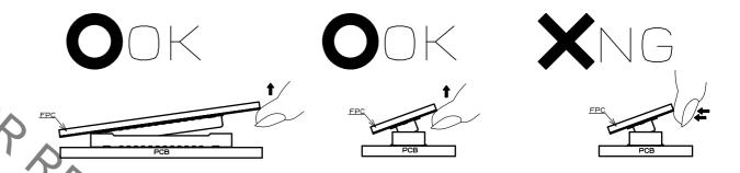
(3) IF THE FPC IS NOT RIGID. THE CONNECTOR CAN BE BROKEN. PLEASE CHECK THE ACTION OF THE FPC TO BE USED REPEATEBLY AT THE TIME OF TRIAL PRODUCTION. BE CAREFUL TO UN-MATE THEM FROM THE PITCH DIRECTION, PULLING IT FROM THE CORNER CAN ALSO RISK TO PUTTING STRESS ON CONTACTS.
