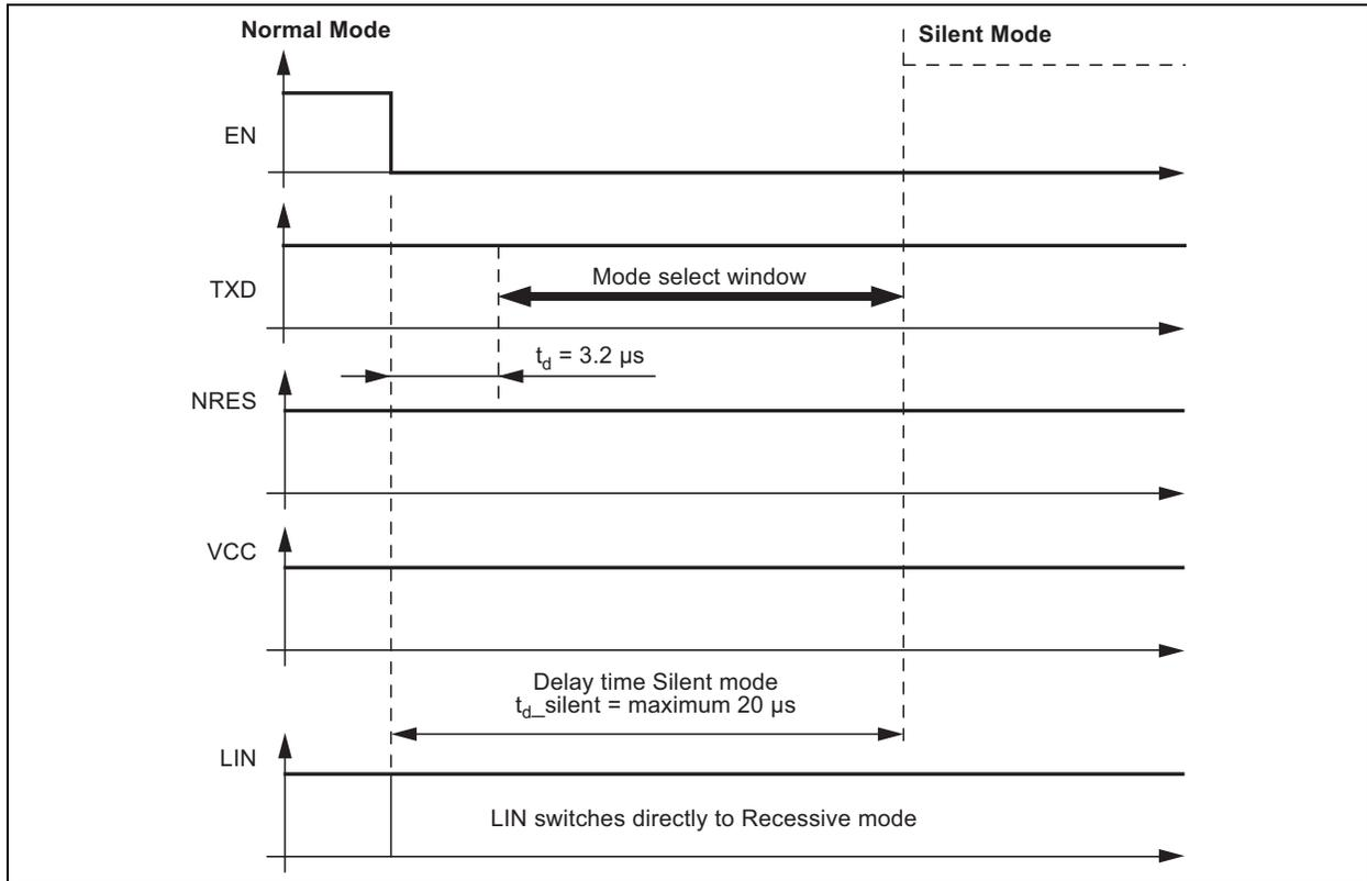
In Silent mode, the internal slave termination between the LIN pin and VS pin is disabled to minimize the current consumption in case the pin LIN is short-circuited to GND. Only a weak pull-up current (typically  $10 \mu A$ ) between the LIN pin and VS pin is present. Silent mode can be activated independently from the current level on pin LIN.
