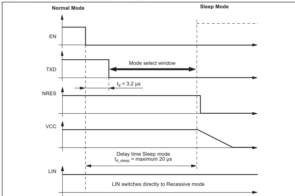
In order to avoid any influence to the LIN pin when switching into Sleep mode, it is possible to switch EN up to  $3.2 \mu\text{s}$  earlier to low than TXD. The easiest and best way to do this is by having two falling edges at TXD and EN at the same time.
