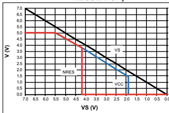
The upper graphs are only valid if the VS ramp-up and ramp-down times are much slower than the VCC ramp-up time  $t_{VCC}$  and the NRES delay time  $t_{reset}$ .
