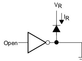
Figure 20.  $I_R$  Test Circuit
