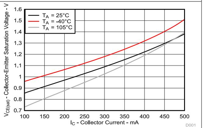
Figure 4. Collector-Emitter Saturation Voltage vs Collector Current
