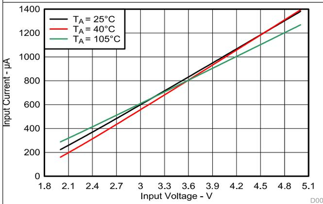
Figure 3. Input Current vs Input Voltage
