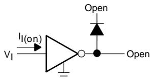
Figure 17.  $I_I$  Test Circuit
