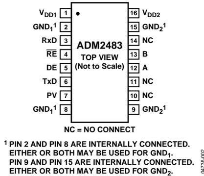
Figure 2. Pin Configuration
