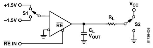
Figure 8. Receiver Enable/Disable
