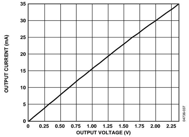
Figure 25. Output Current vs. Receiver Output Low Voltage
