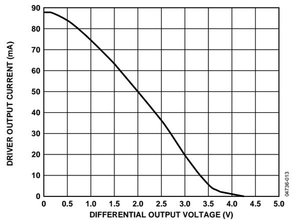
Figure 18. Driver Output Current vs. Differential Output Voltage
