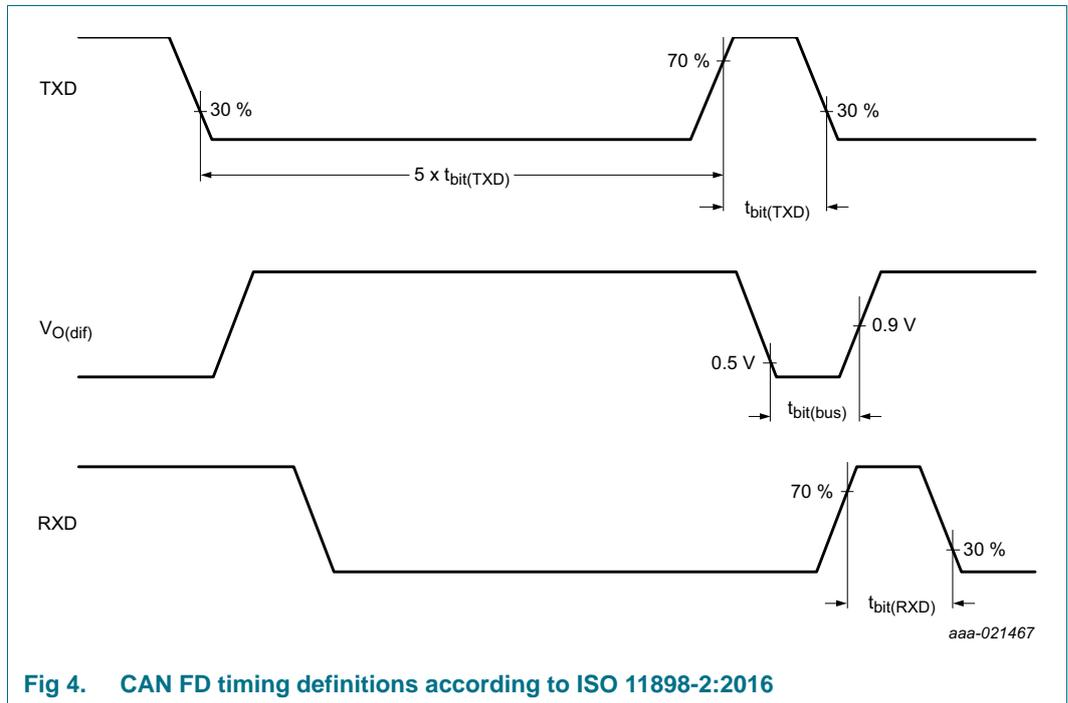
Fig 4. CAN FD timing definitions according to ISO 11898-2:2016
