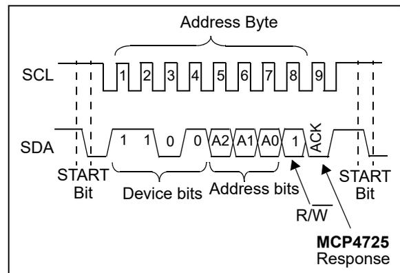
**FIGURE 8-2:** I<sup>2</sup>C Bus Connection Test.
