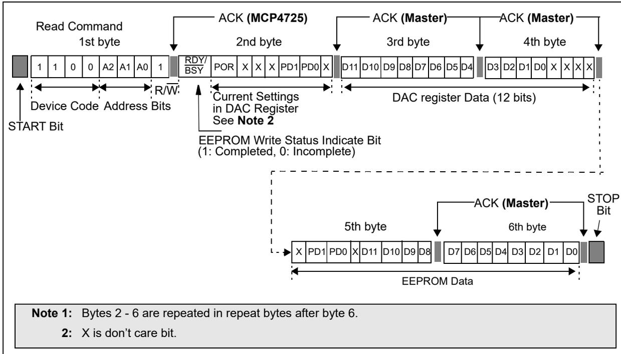
FIGURE 6-3: Read Command and Output Data Format.
