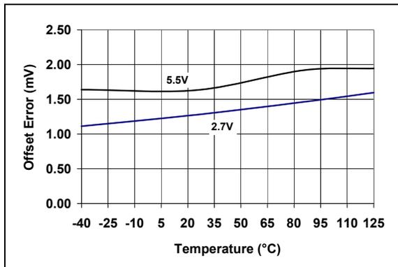
**FIGURE 2-14:** Offset Error vs. Temperature and  $V_{DD}$ .
