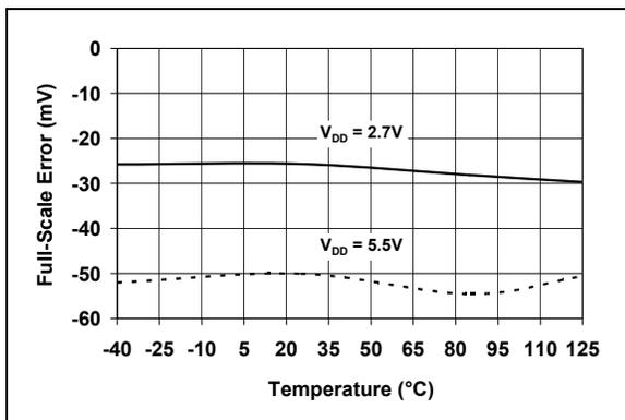
**FIGURE 2-9:** Full Scale Error vs. Temperature (Code = 4095d).
