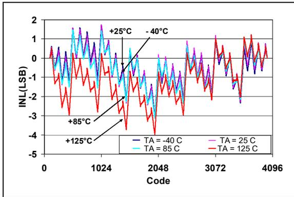
**FIGURE 2-7:** INL vs. Code and Temperature ( $V_{DD} = 2.7\text{V}$ ).
