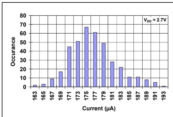
**FIGURE 2-13:**  $I_{DD}$  Histogram.
