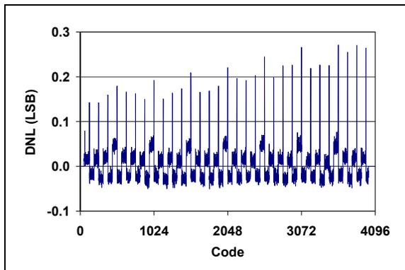
**FIGURE 2-3:** DNL vs. Code ( $V_{DD} = 2.7\text{V}$ ).
