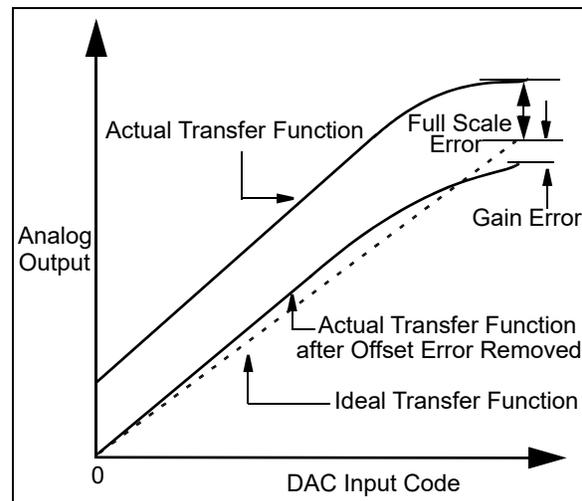
**FIGURE 4-4:** Gain Error and Full Scale Error.
