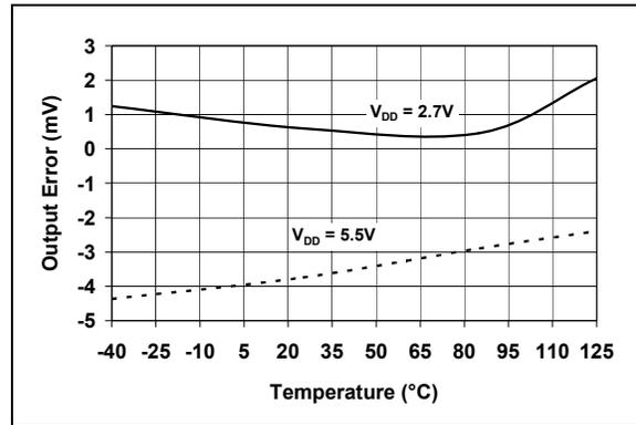
**FIGURE 2-10:** Output Error vs. Temperature (Code = 4000d).
