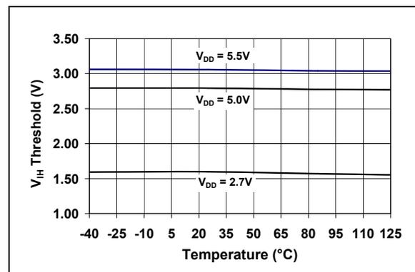
**FIGURE 2-17:**  $V_{IN}$  High Threshold vs. Temperature and  $V_{DD}$ .
