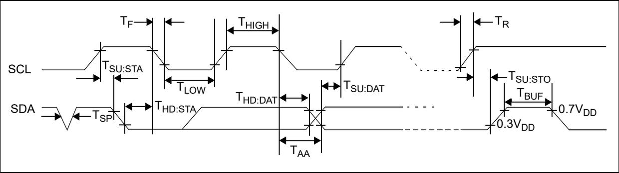
FIGURE 7-4: I<sup>2</sup>C Bus Timing Data.
