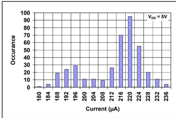
**FIGURE 2-12:**  $I_{DD}$  Histogram.
