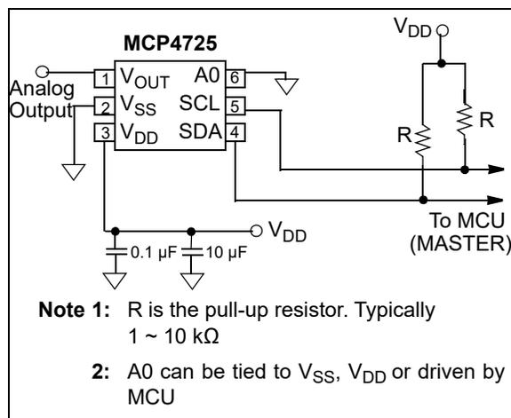
**FIGURE 8-1:** I<sup>2</sup>C Bus Interface Connection with A0 pin tied to V<sub>SS</sub>.
