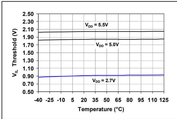
**FIGURE 2-18:**  $V_{IN}$  Low Threshold vs. Temperature and  $V_{DD}$ .
