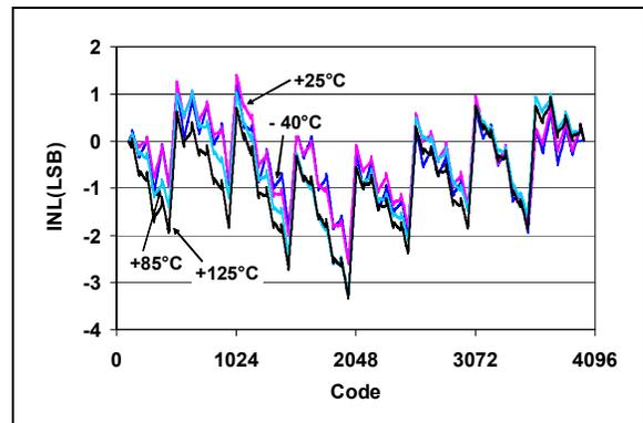
**FIGURE 2-6:** INL vs. Code and Temperature ( $V_{DD} = 5.5\text{V}$ ).
