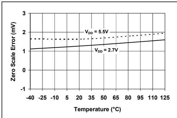
**FIGURE 2-8:** Zero Scale Error vs. Temperature (Code = 000d).
