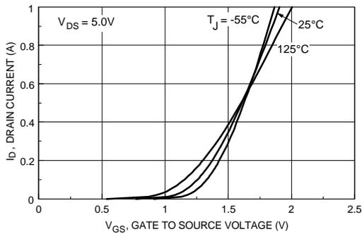
Figure 5. Transfer Characteristics.
