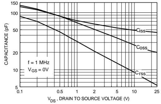
Figure 8. Capacitance Characteristics.
