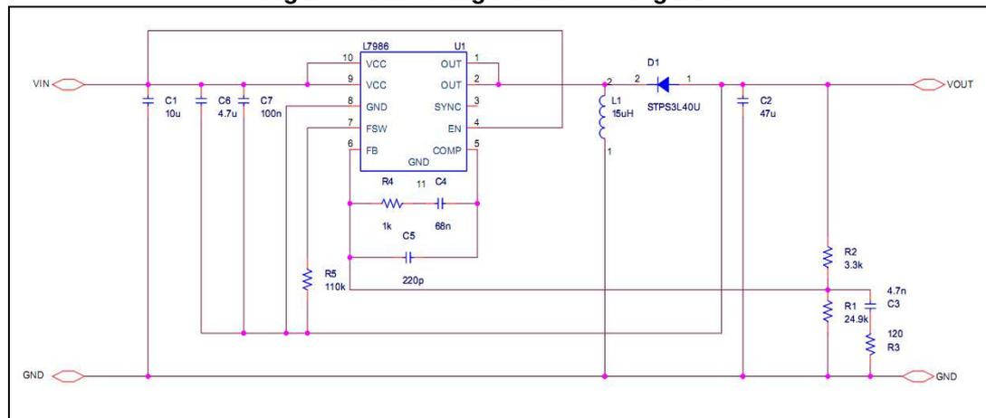
The GND pin of the device is connected to the output voltage so, given the output voltage, the input voltage range is limited by the maximum voltage the device can withstand across VCC and GND (38 V). Therefore, if the output is -5 V the input voltage can range from 4.5 V to 33 V.
