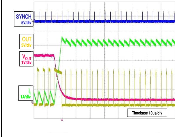
Figure 33. Short-circuit behavior  $V_{in} = 24 V$
