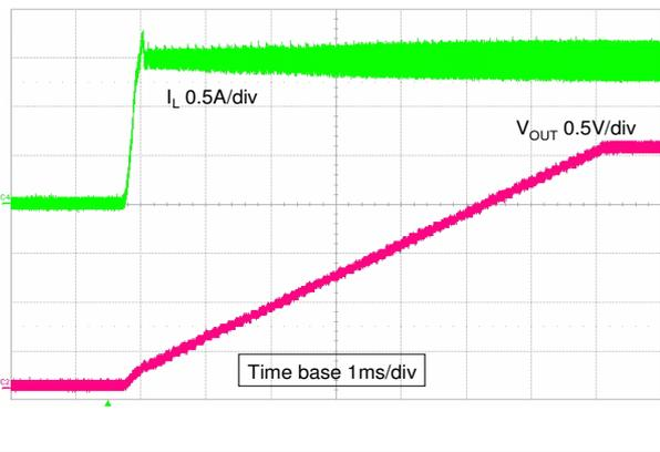
Figure 32. Short-circuit behavior  $V_{in} = 12 V$
