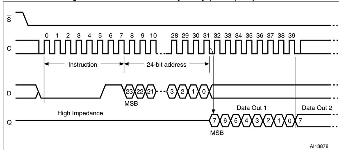
If Chip Select ( $\bar{S}$ ) continues to be driven low, the internal address register is incremented automatically, and the byte of data at the new address is shifted out.
