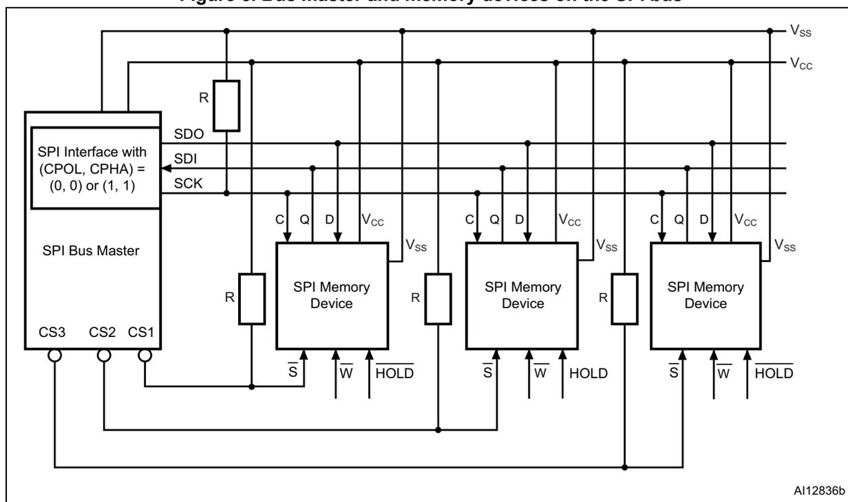
1. The Write Protect ( $\bar{W}$ ) and Hold ( $\overline{HOLD}$ ) signals should be driven, high or low as appropriate.
