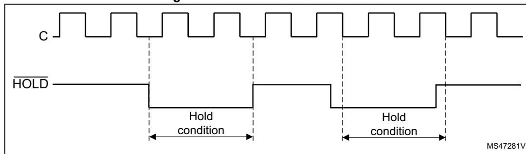
The Hold condition starts when the Hold ( $\overline{HOLD}$ ) signal is driven low when Serial Clock (C) is already low (as shown in [Figure 7](#)).
