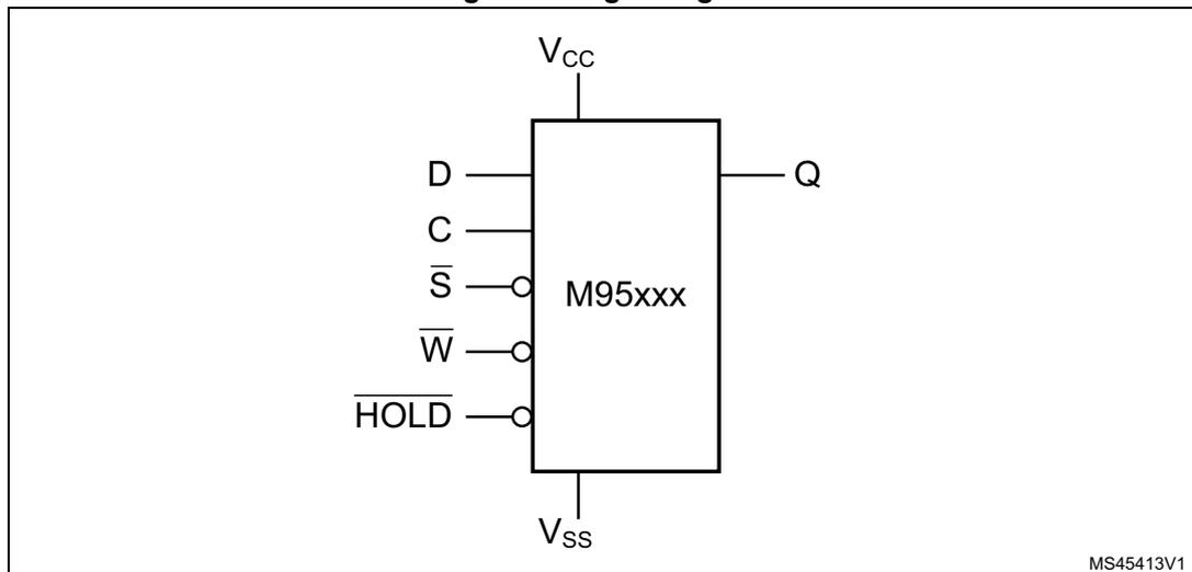
The SPI bus signals are C, D and Q, as shown in [Figure 1](#) and [Table 1](#). The device is selected when Chip Select ( $\overline{S}$ ) is driven low. Communications with the device can be interrupted when the HOLD is driven low.
