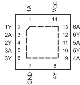
Figure 5-2. RGY Package, 14-Pin VQFN (Top View)
