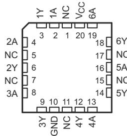
Figure 5-3. FK Package, 20-Pin LCCC (Top View)
