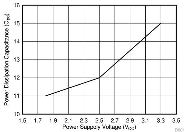
**Figure 6-1. Power Dissipation Capacitance vs. Power Supply Voltage**
