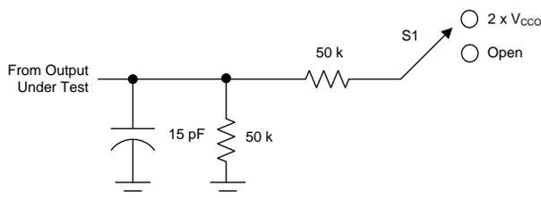
**Figure 6. Load Circuit For Enable / Disable Time Measurement**
