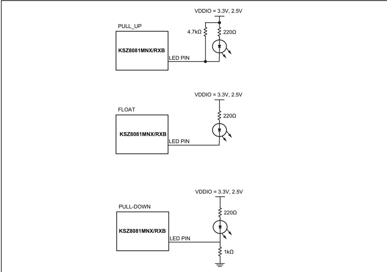
For using 1.8V VDDIO, should select parts with low 1.8V operation voltage and forwarding current  $I_F$  about 2 mA LED indicator. It is okay to use internal pull-up or external pull-up resistor for the LED pin pull-up strap function, and use an external 0.75 kΩ to 1 kΩ pull-down resistor for the LED pin pull-down strap function.
