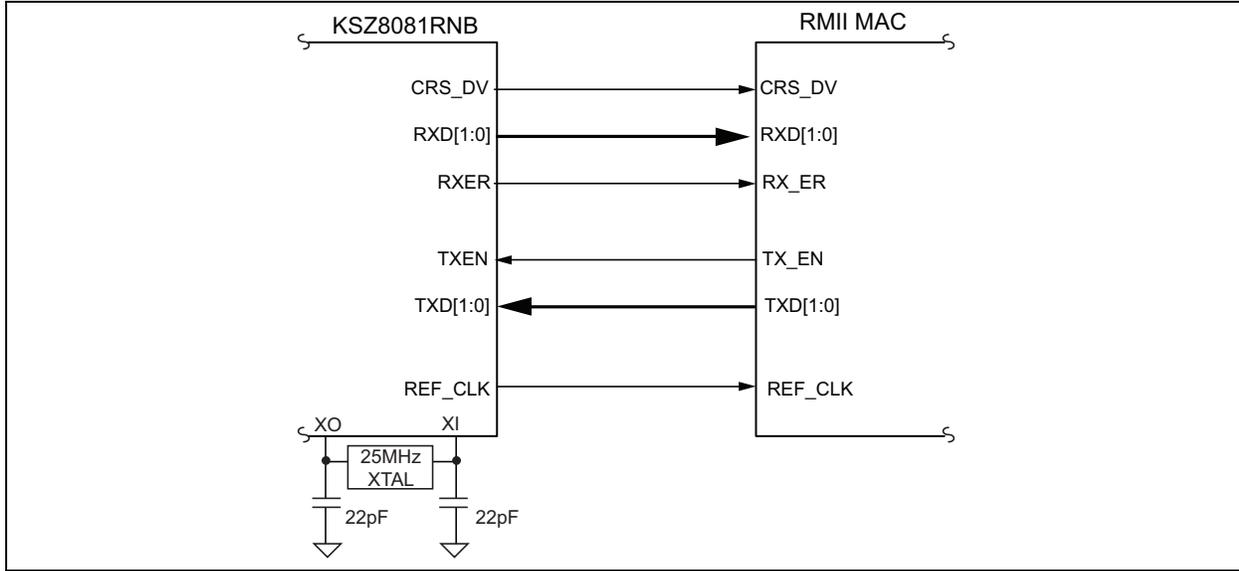
**FIGURE 3-4: KSZ8081RNB RMII INTERFACE (50 MHZ CLOCK MODE)**
