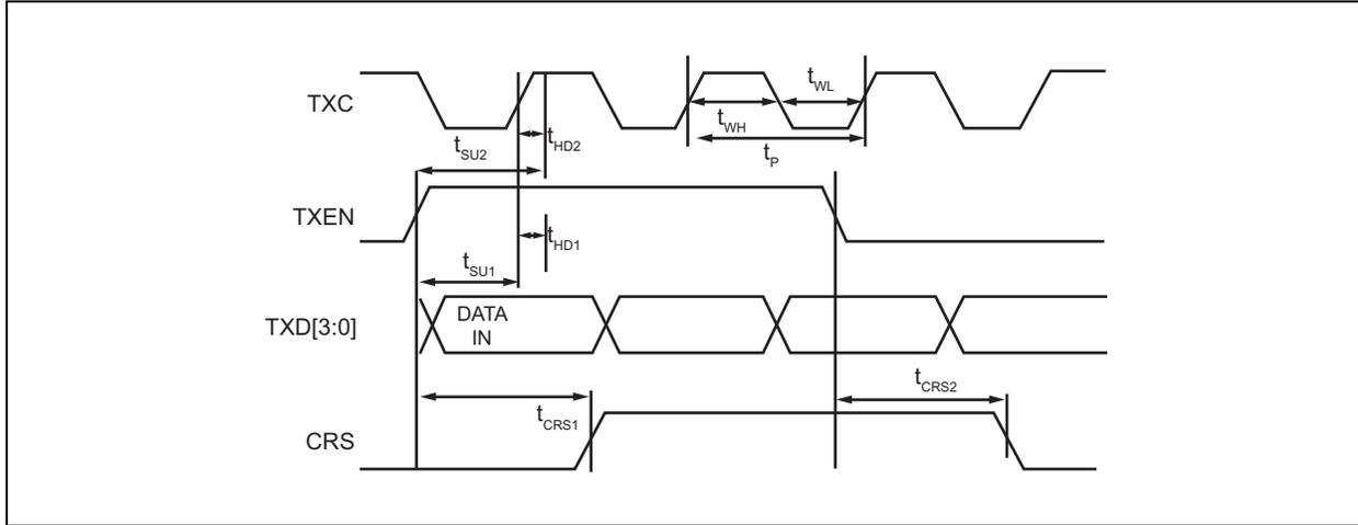
TABLE 7-4: MII TRANSMIT TIMING (BASE100BASE-TX) PARAMETERS
