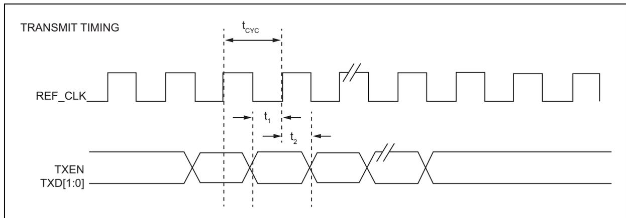
**FIGURE 7-7: RMII TIMING – DATA INPUT TO RMII**
