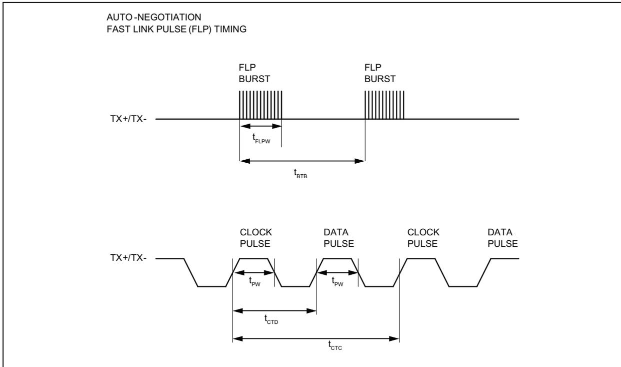
**TABLE 7-8: AUTO-NEGOTIATION FAST LINK PULSE (FLP) TIMING PARAMETERS**
