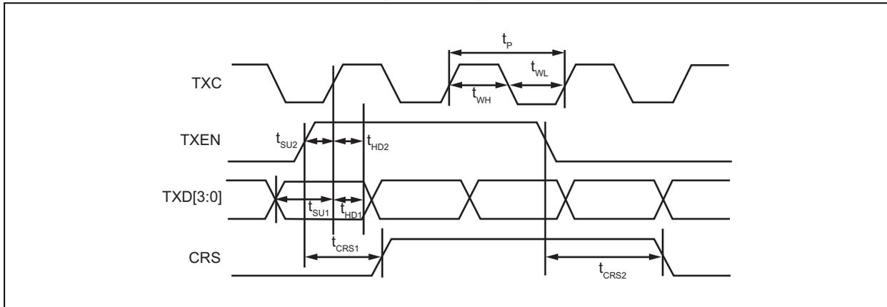
TABLE 7-2: MII TRANSMIT TIMING (10BASE-T) PARAMETERS
