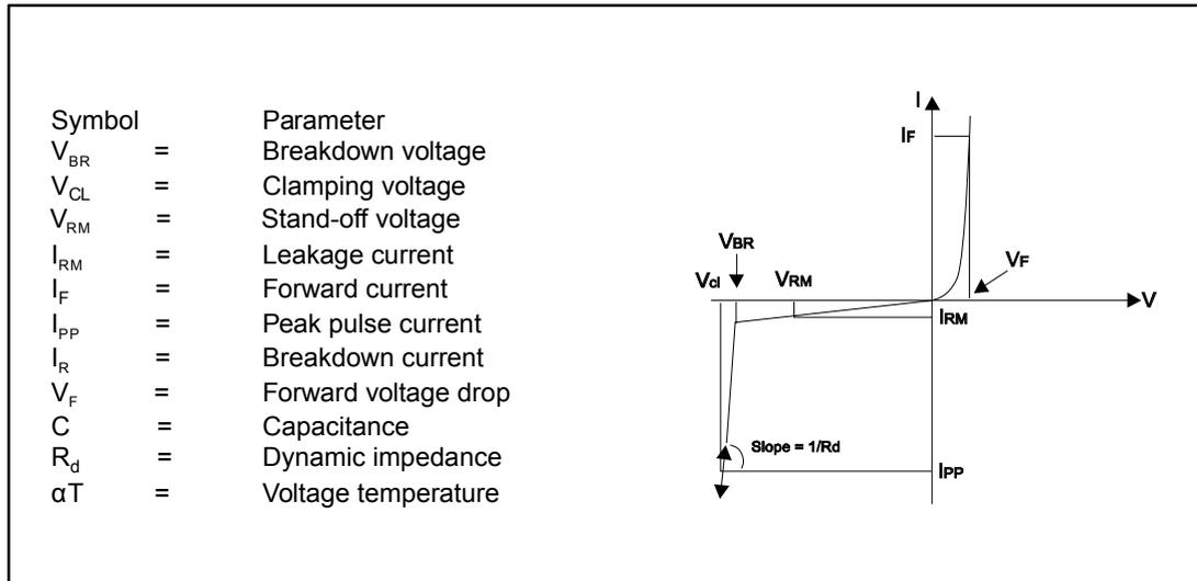
Table 2: Electrical characteristics ( $T_{amb} = 25\text{ °C}$ )
