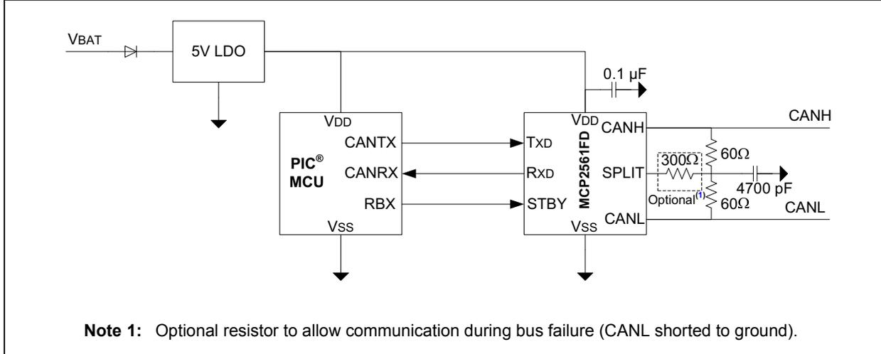
**FIGURE 1-2: MCP2562FD WITH V<sub>IO</sub> PIN**
