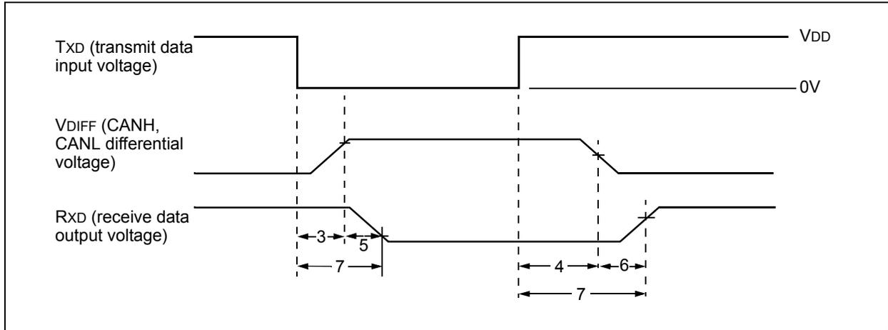
**FIGURE 2-8: TIMING DIAGRAM FOR WAKEUP FROM STANDBY**
