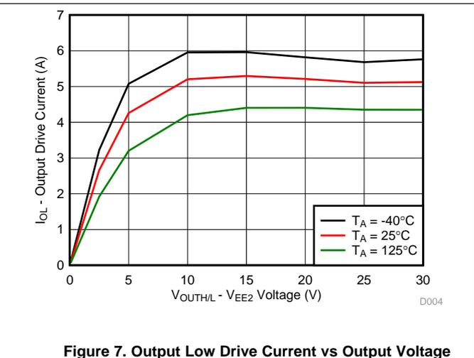
Figure 7. Output Low Drive Current vs Output Voltage
