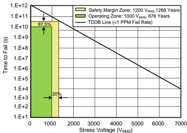
$T_A$  up to 150°C Stress-voltage frequency = 60 Hz
