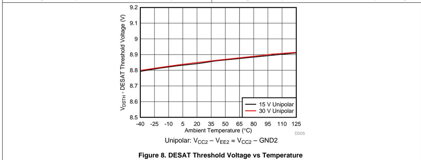
Figure 8. DESAT Threshold Voltage vs Temperature
