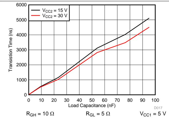
Figure 30.  $t_r$  Rise Time vs Load Capacitance
