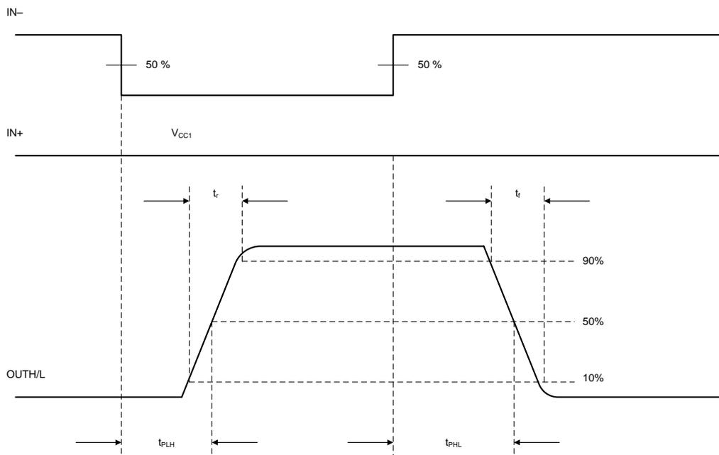
Figure 45. OUTH and OUTL Propagation Delay, Inverting Configuration
