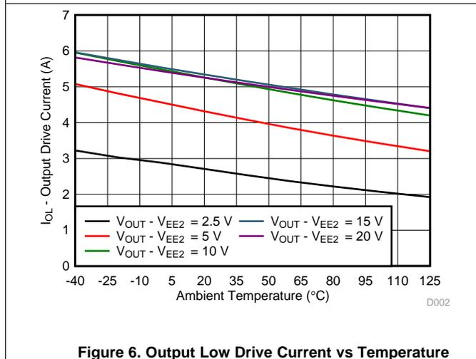
Figure 6. Output Low Drive Current vs Temperature
