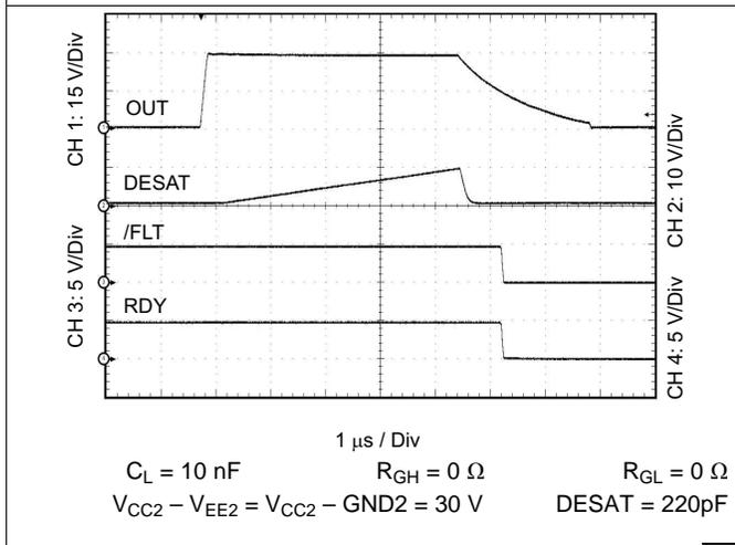
Figure 17. Output Transient Waveform DESAT, RDY and FLT
