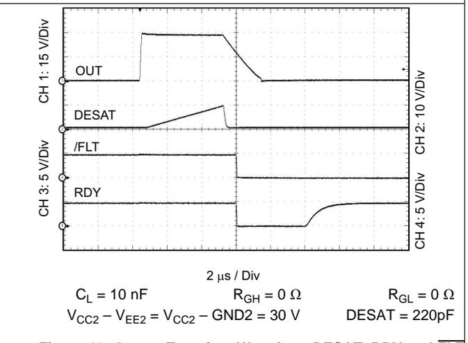
Figure 18. Output Transient Waveform DESAT, RDY and FLT
