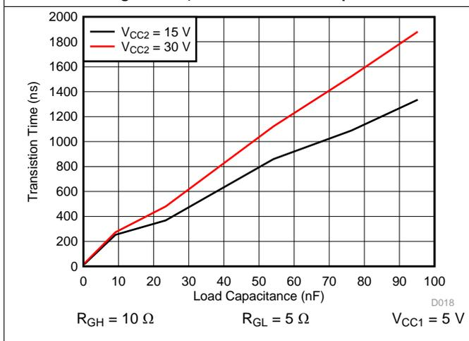
Figure 31.  $t_f$  Fall Time vs Load Capacitance
