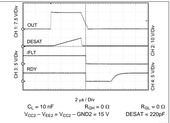
Figure 16. Output Transient Waveform DESAT, RDY and FLT
