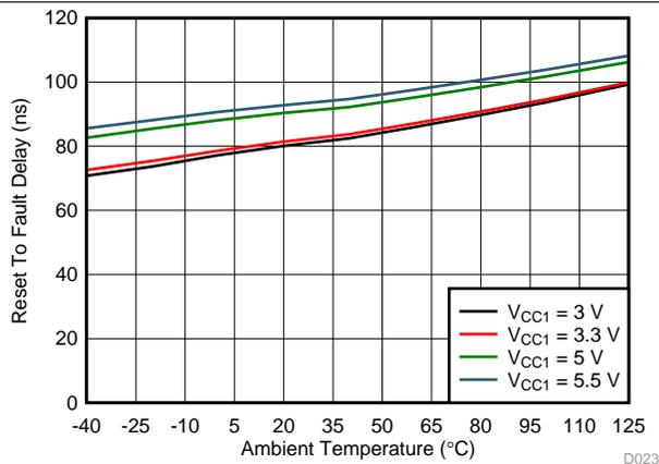
Figure 37. Reset to Fault Delay Across Temperature
