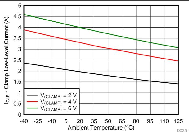
Figure 38. Miller Clamp Current vs Temperature
