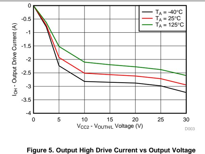
Figure 5. Output High Drive Current vs Output Voltage
