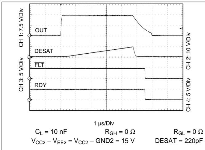
Figure 15. Output Transient Waveform DESAT, RDY and FLT
