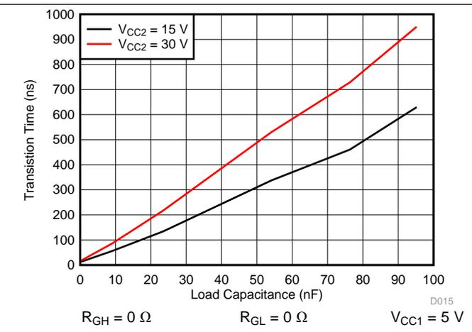
Figure 28.  $t_r$  Rise Time vs Load Capacitance
