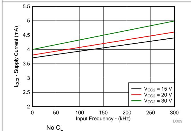
Figure 23.  $I_{CC2}$  Supply Current vs Input Frequency
