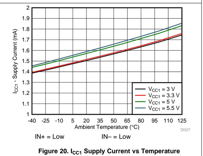
Figure 20.  $I_{CC1}$  Supply Current vs Temperature
