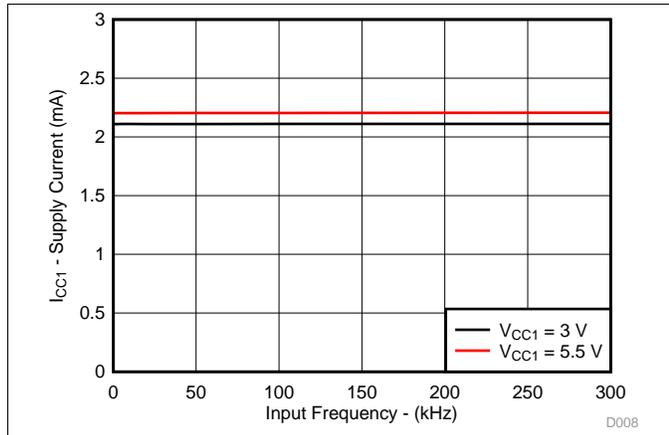
Figure 21.  $I_{CC1}$  Supply Current vs Input Frequency
