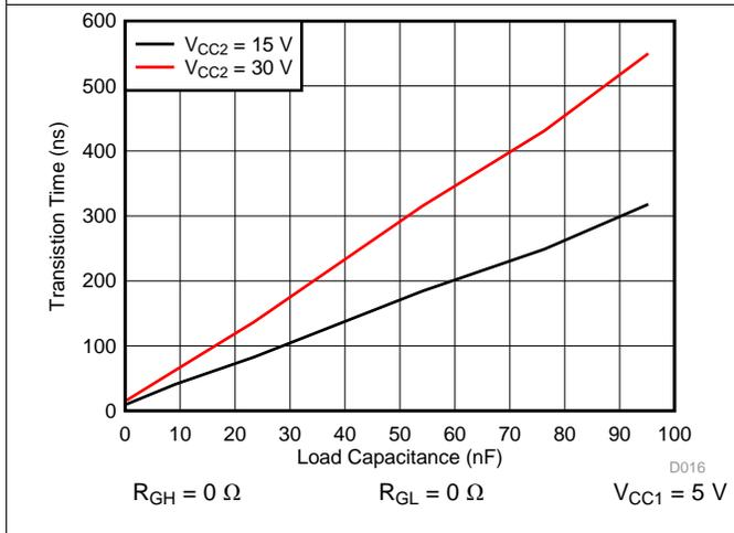
Figure 29.  $t_f$  Fall Time v. Load Capacitance
