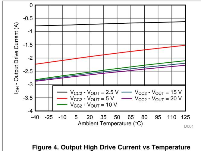
Figure 4. Output High Drive Current vs Temperature
