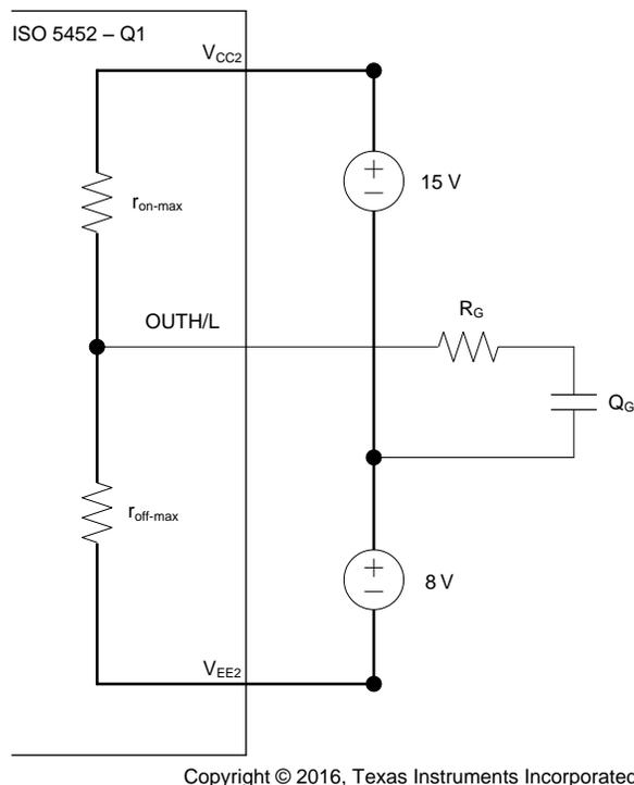
**Figure 56. Simplified Output Model for Calculating  $P_{OL-WC}$**
