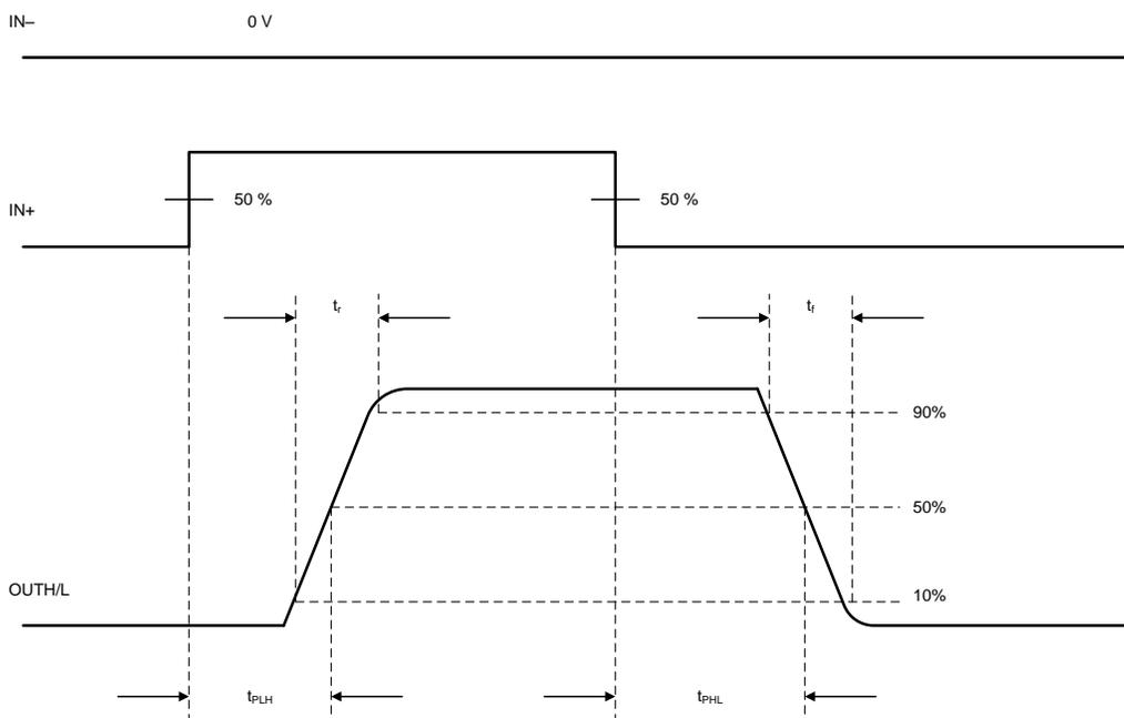
Figure 44. OUTH and OUTL Propagation Delay, Noninverting Configuration
