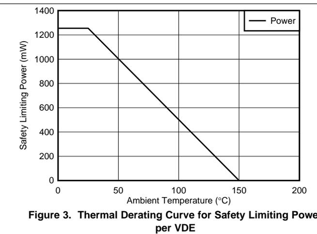
**Figure 3. Thermal Derating Curve for Safety Limiting Power per VDE**
