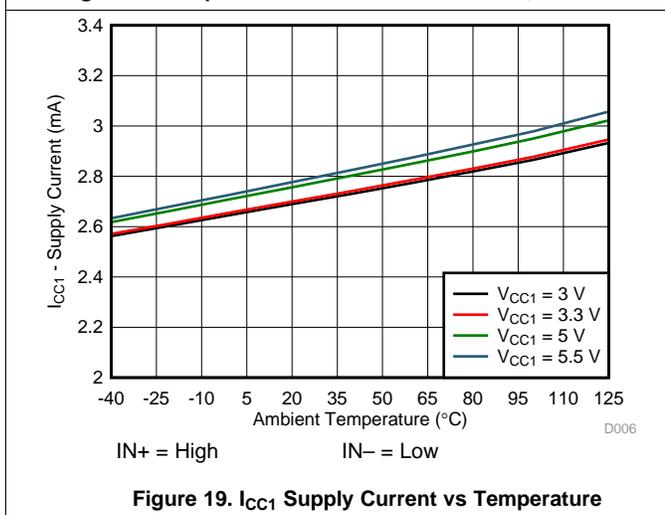
Figure 19.  $I_{CC1}$  Supply Current vs Temperature
