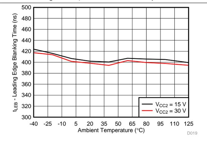
Figure 32. Leading Edge Blanking Time With Temperature
