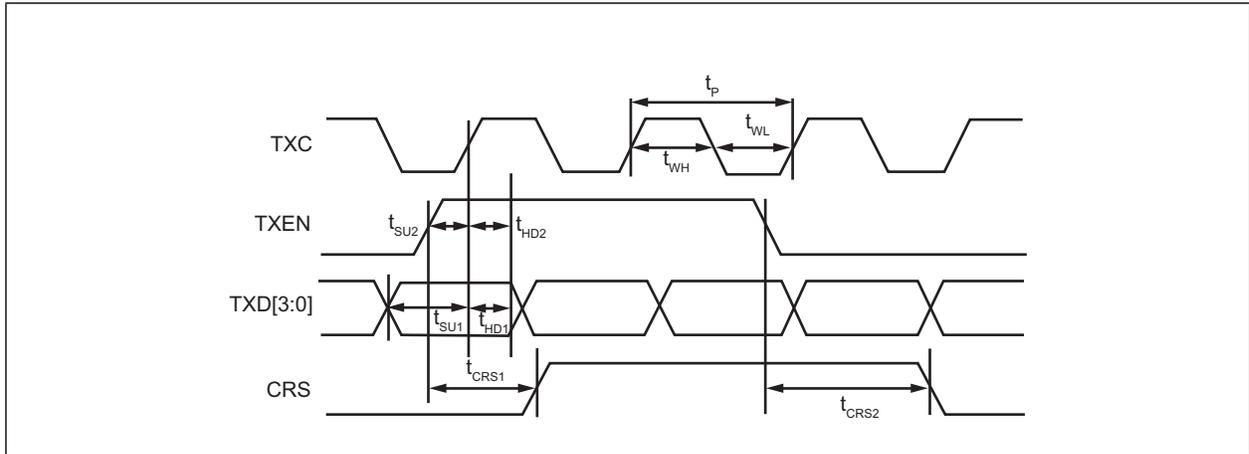
TABLE 7-2: MII TRANSMIT TIMING (10BASE-T) PARAMETERS
