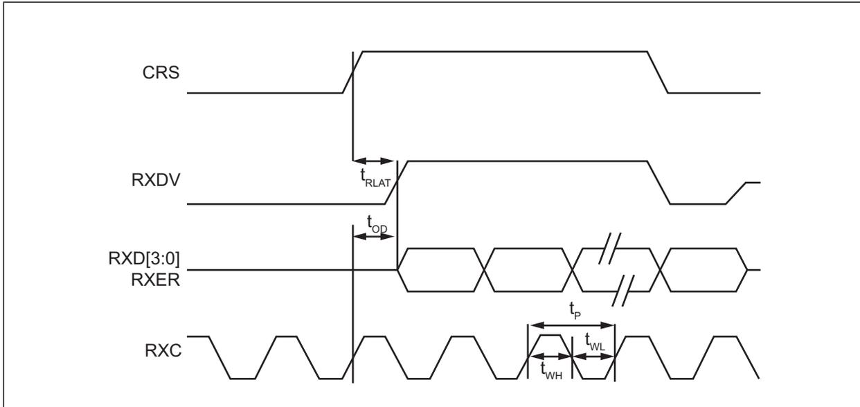
TABLE 7-3: MII RECEIVE TIMING (10BASE-T) PARAMETERS
