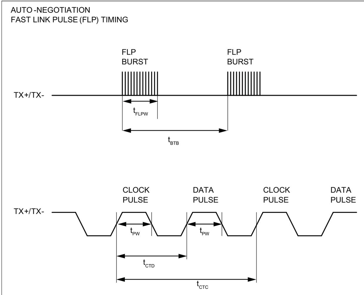
**TABLE 7-8: AUTO-NEGOTIATION FAST LINK PULSE TIMING PARAMETERS**
