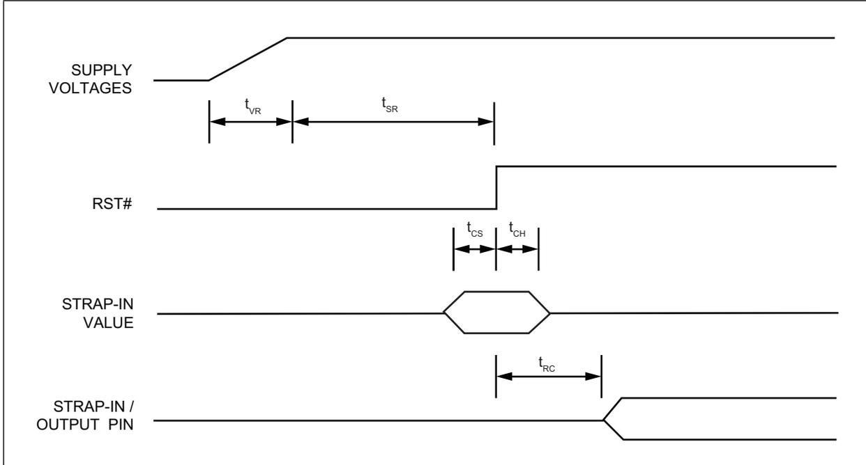
**TABLE 7-10: POWER-UP/RESET TIMING PARAMETERS**
