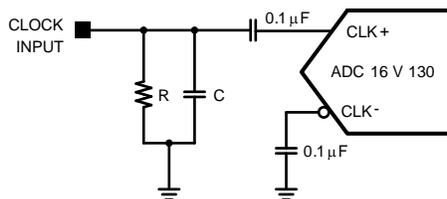
Figure 27. Singled-Ended 1.8V Clocking, Capacitive AC Coupled
