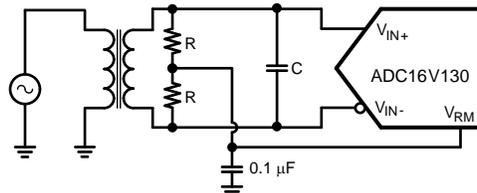
**Figure 21. Transformer Drive Circuit for Low Input Frequency**
