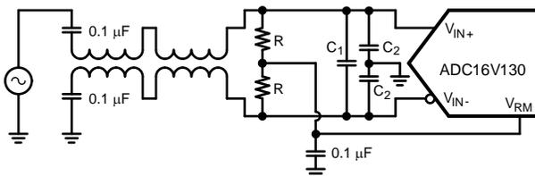
Figure 22. Transformer Drive Circuit for High Input Frequency
