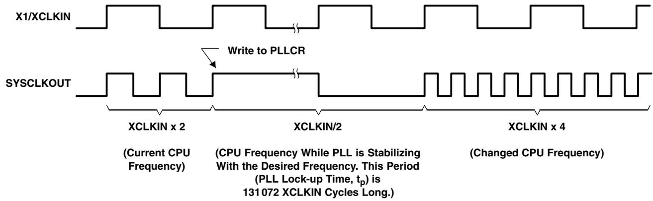
Figure 6–11. Effect of Writing Into PLLCR Register
