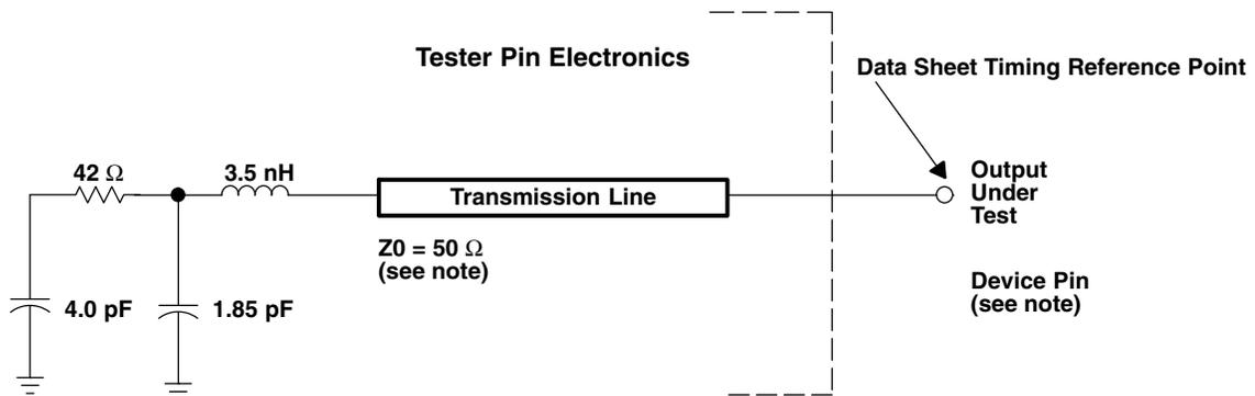
NOTE: The data sheet provides timing at the device pin. For output timing analysis, the tester pin electronics and its transmission line effects must be taken into account. A transmission line with a delay of 2 ns or longer can be used to produce the desired transmission line effect. The transmission line is intended as a load only. It is not necessary to add or subtract the transmission line delay (2 ns or longer) from the data sheet timing.
