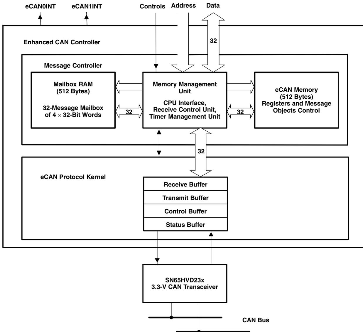
Figure 4-7. eCAN Block Diagram and Interface Circuit
