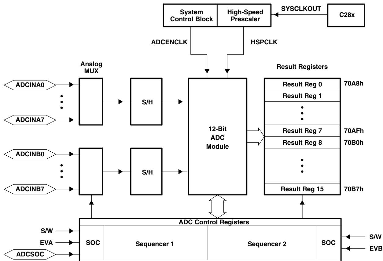
Figure 4-4. Block Diagram of the F2812 ADC Module
