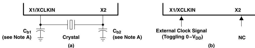
NOTE A: TI recommends that customers have the resonator/crystal vendor characterize the operation of their device with the DSP chip. The resonator/crystal vendor has the equipment and expertise to tune the tank circuit. The vendor can also advise the customer regarding the proper tank component values that ensures start-up and stability over the entire operating range.
