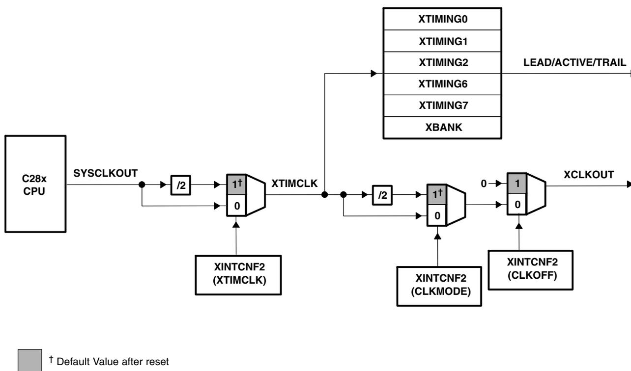
**Figure 6–27. Relationship Between XTIMCLK and SYSCLKOUT**
