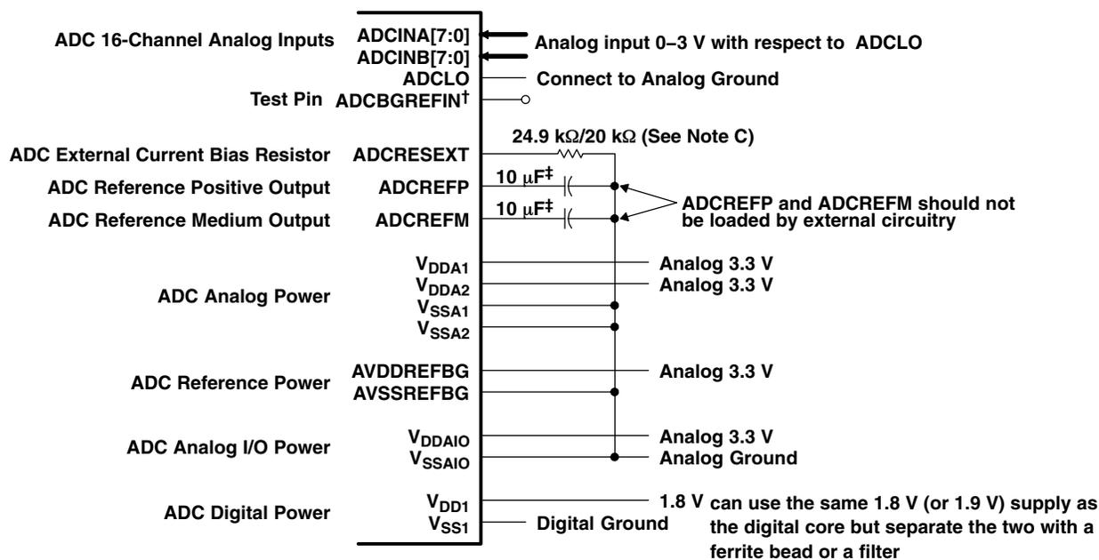
† Provide access to this pin in PCB layouts. Intended for test purposes only.
