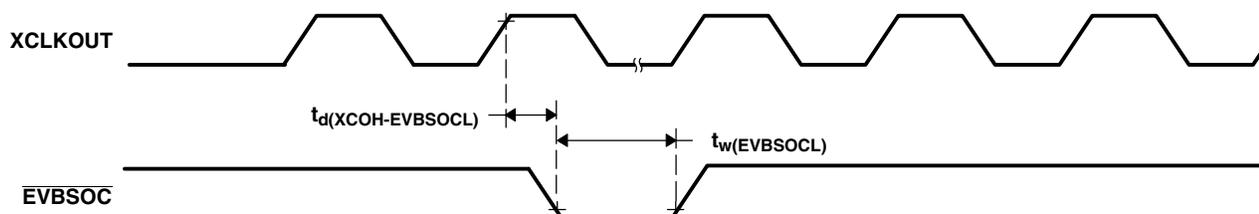
**Figure 6–18. EVBSOC Timing**
