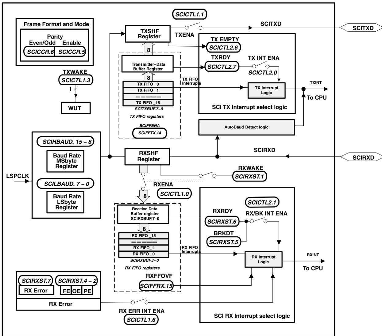
Figure 4–10. Serial Communications Interface (SCI) Module Block Diagram
