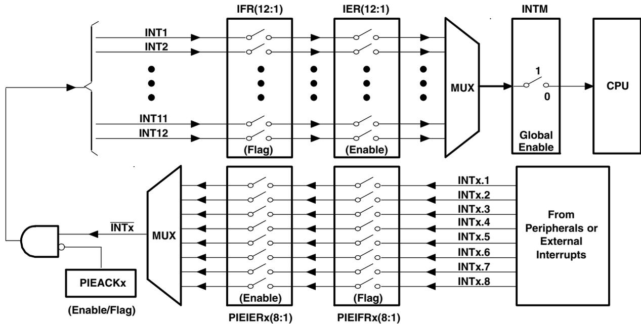
Figure 3–5. Multiplexing of Interrupts Using the PIE Block
