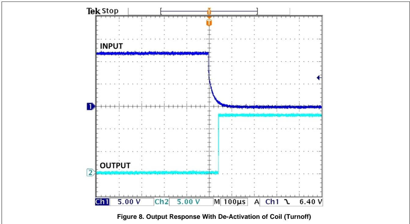
Figure 8. Output Response With De-Activation of Coil (Turnoff)
