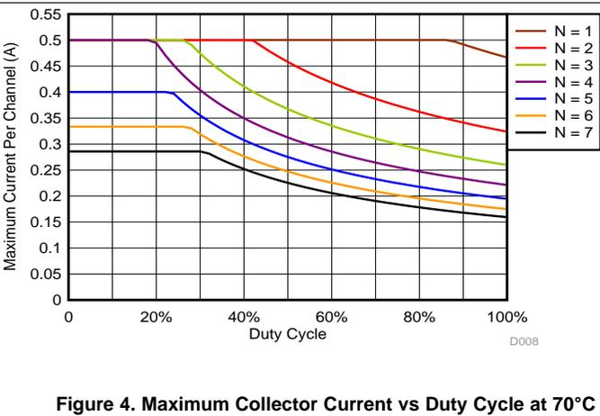
**Figure 4. Maximum Collector Current vs Duty Cycle at 70°C**
