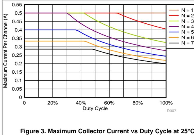
**Figure 3. Maximum Collector Current vs Duty Cycle at 25°C**
