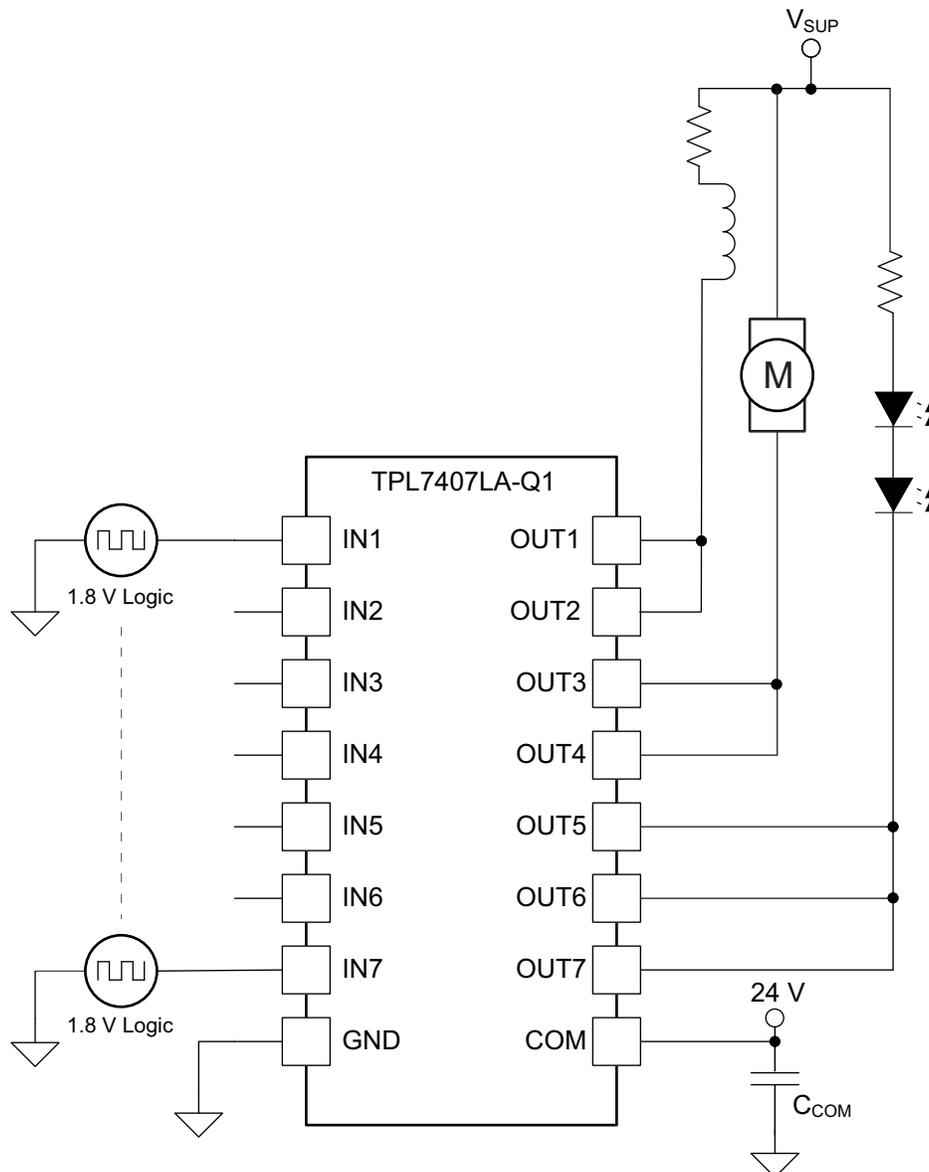
**Figure 6. Multi-Purpose Sink Driver Schematic**
