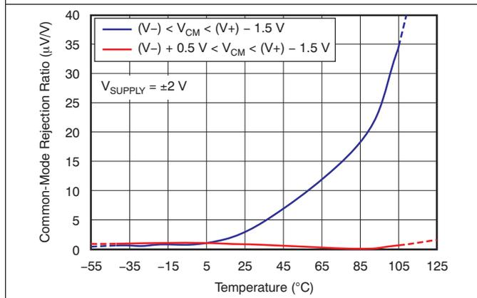
Figure 11. CMRR vs Temperature
