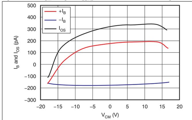
Figure 7.  $I_B$  and  $I_{OS}$  vs Common-Mode Voltage
