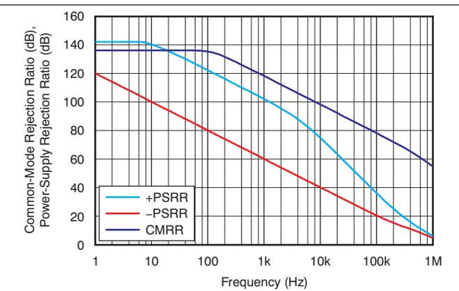
Figure 10. CMRR and PSRR vs Frequency (Referred-to-Input)
