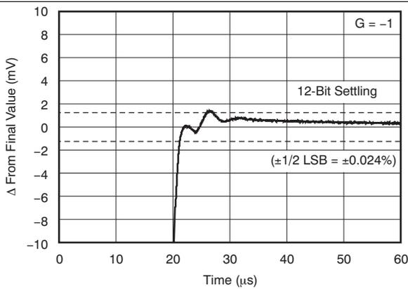
Figure 33. Large-Signal Settling Time (10-V Positive Step)
