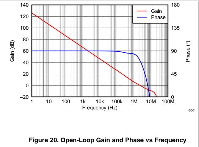
Figure 20. Open-Loop Gain and Phase vs Frequency
