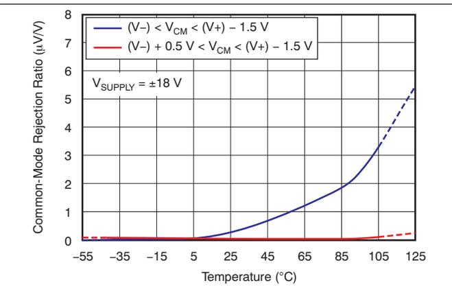
Figure 12. CMRR vs Temperature
