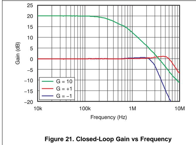
Figure 21. Closed-Loop Gain vs Frequency
