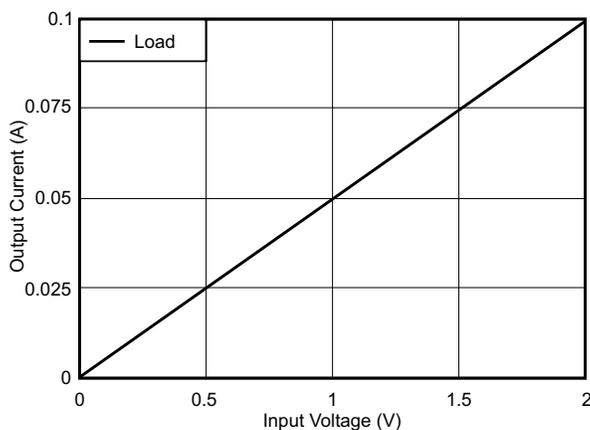
**Figure 45. Measured Transfer Function for High-Side V-I Converter**
