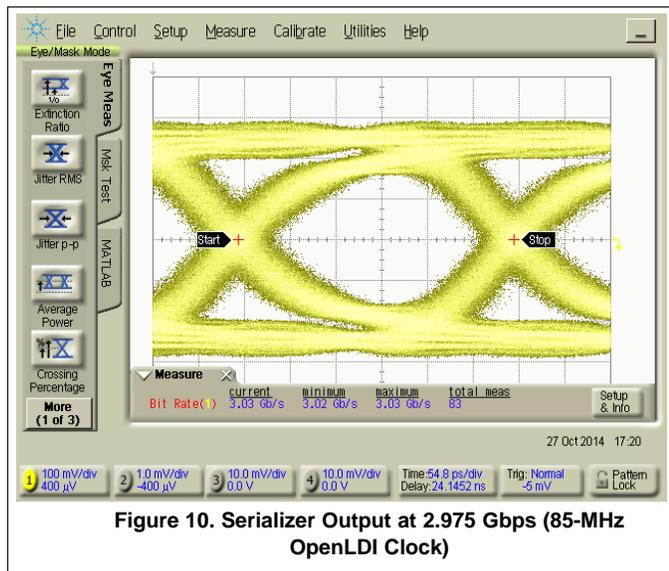
Figure 10. Serializer Output at 2.975 Gbps (85-MHz OpenLDI Clock)
