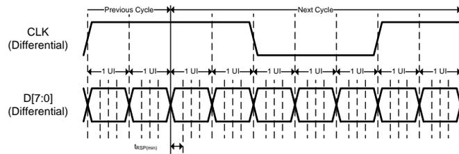
Figure 3. OpenLDI Input Clock and Data Jitter
