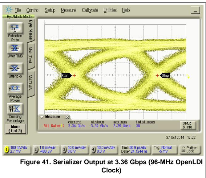
Figure 41. Serializer Output at 3.36 Gbps (96-MHz OpenLDI Clock)
