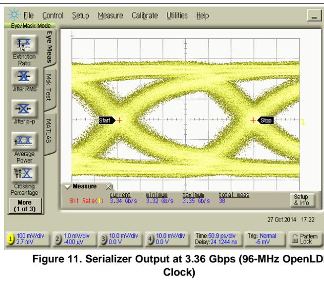
Figure 11. Serializer Output at 3.36 Gbps (96-MHz OpenLDI Clock)
