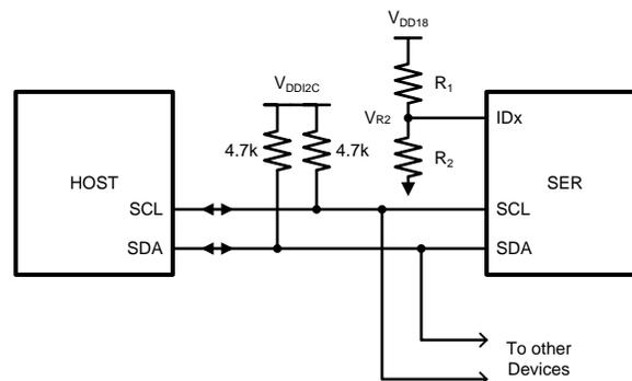
Figure 31. Serial Control Bus Connection
