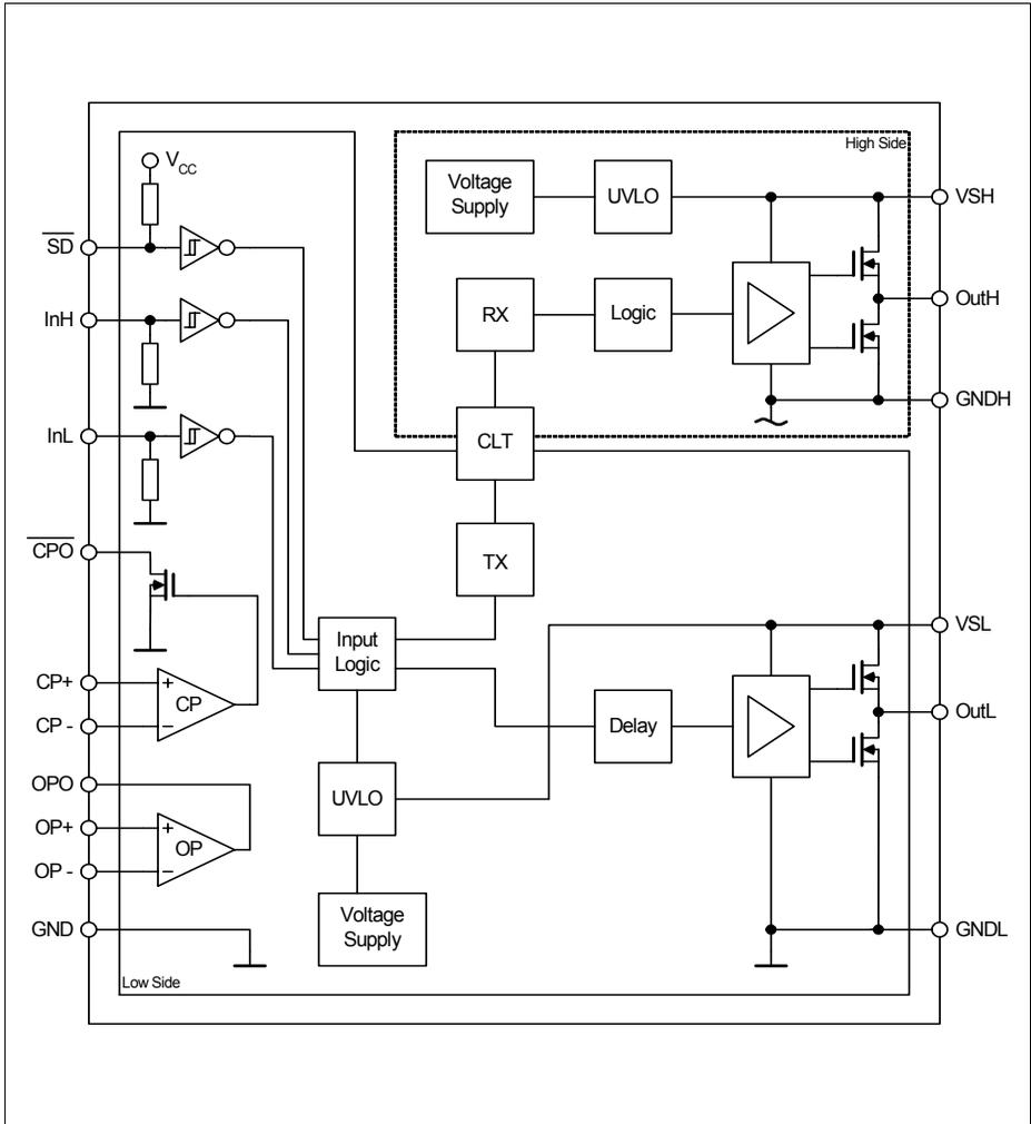
Figure 2 Block Diagram
