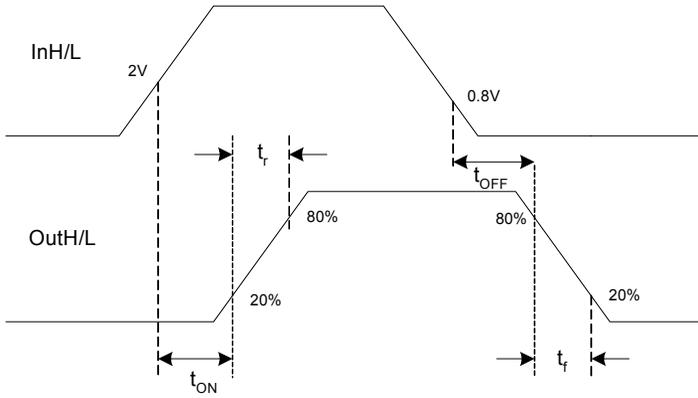
Figure 4 Switching Time Waveform Definition
