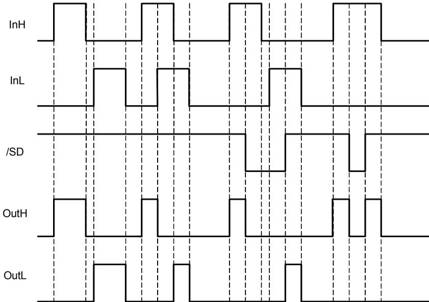
Figure 3 Input/Output Timing Diagram
