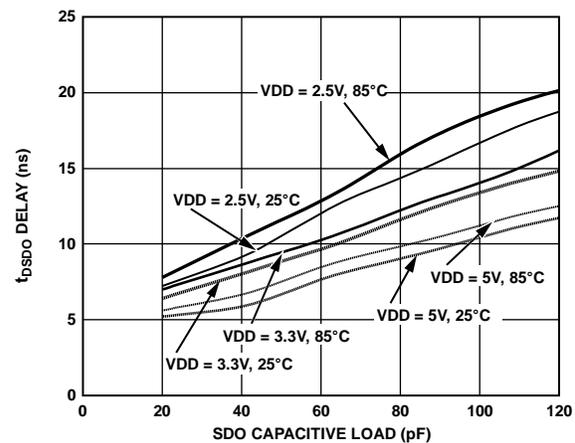
Figure 24.  $t_{psdc}$  Delay vs. Capacitance Load and Supply
