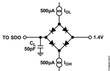
Figure 3. Load Circuit for Digital Interface Timing
