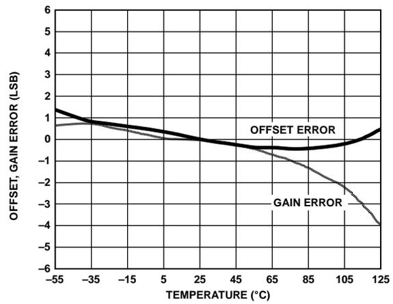
Figure 23. Offset and Gain Error vs. Temperature
