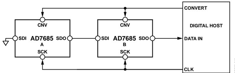
Figure 42. Chain Mode Connection Diagram
