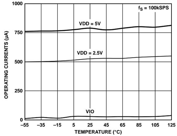
Figure 22. Operating Currents vs. Temperature
