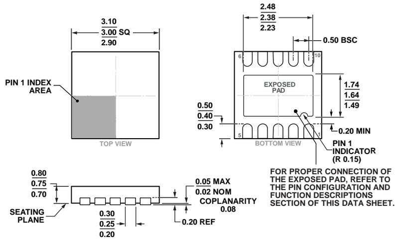
Figure 50. 10-Lead Lead Frame Chip Scale Package [LFCSF\_WD]
