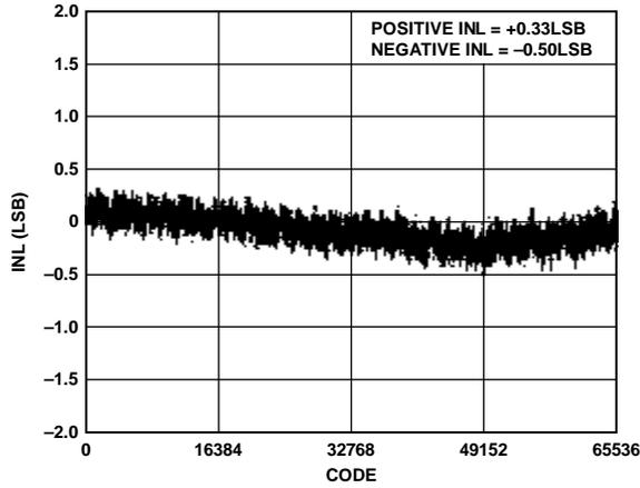
Figure 7. Integral Nonlinearity vs. Code
