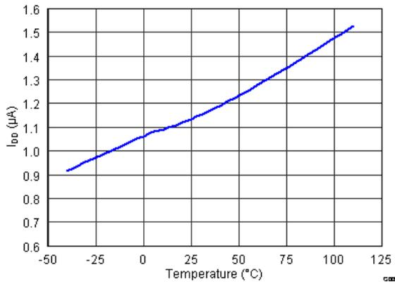
**Figure 9-6. I<sub>DD</sub> Current Consumption vs. Temperature at V<sub>DD</sub> = 16 V**
