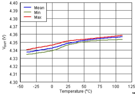
**Figure 7-1. Overvoltage Threshold (Nominal = 4.35 V) vs. Temperature**
