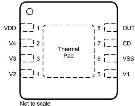
**Figure 6-1. DSG Package 8-Pin WSON Top View**
