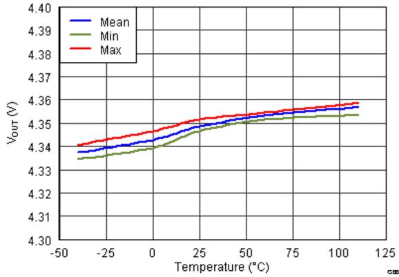
**Figure 9-4. Overvoltage Threshold (OVT) vs. Temperature**
