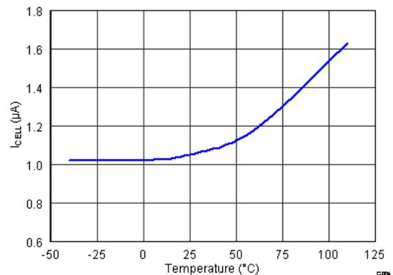
**Figure 7-4.  $I_{\text{CELL}}$  vs. Temperature at  $V_{\text{CELL}} = 9.2\text{V}$**
