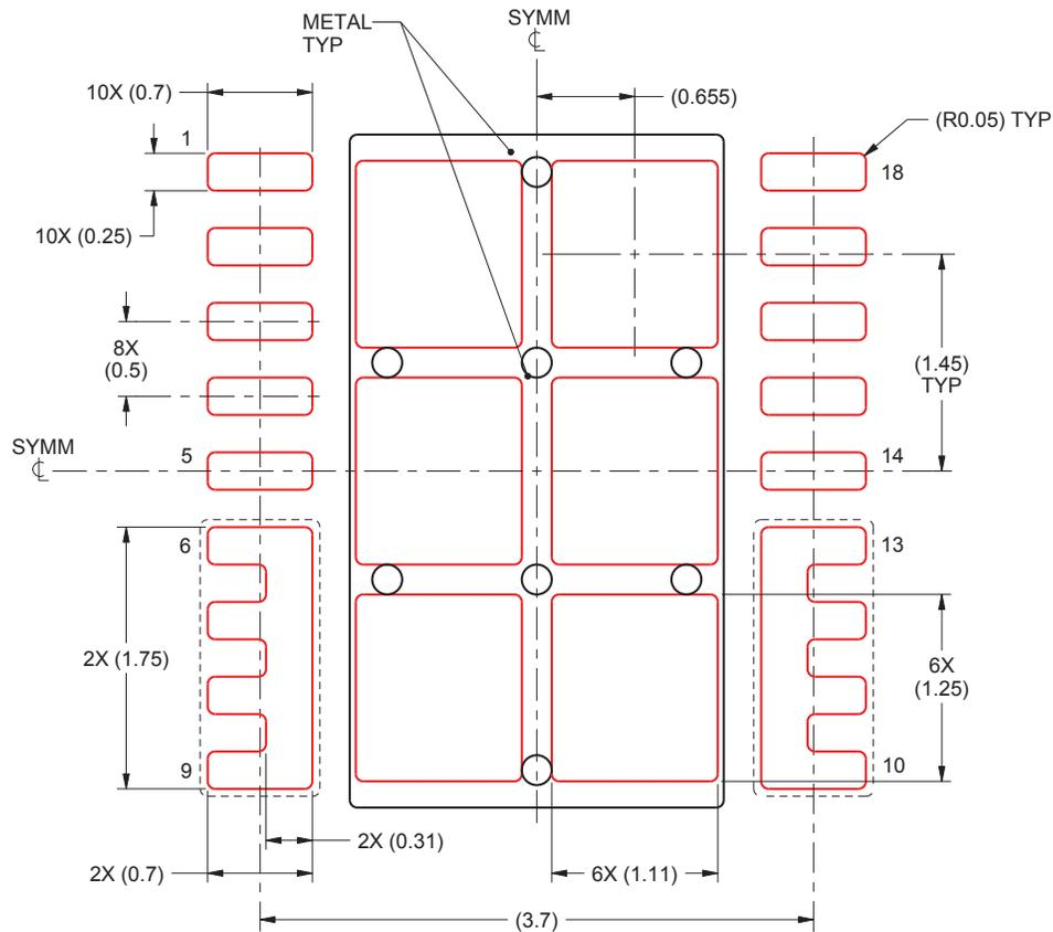
1. All linear dimensions are in millimeters. Any dimensions in parenthesis are for reference only. Dimensioning and tolerancing per ASME Y14.5M.
