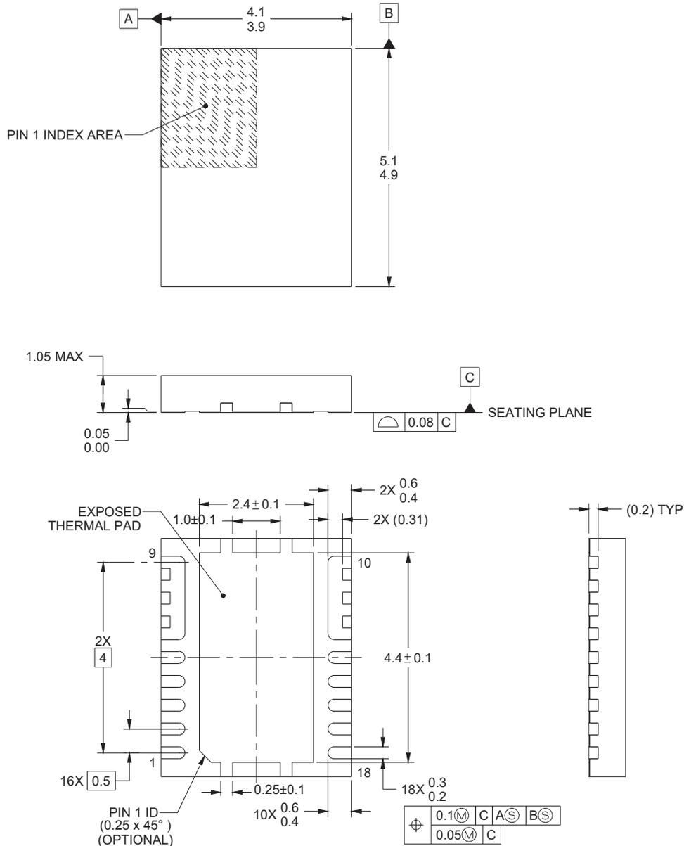
1. All linear dimensions are in millimeters. Any dimensions in parenthesis are for reference only. Dimensioning and tolerancing per ASME Y14.5M.
