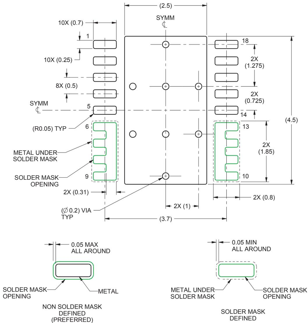
1. All linear dimensions are in millimeters. Any dimensions in parenthesis are for reference only. Dimensioning and tolerancing per ASME Y14.5M.
