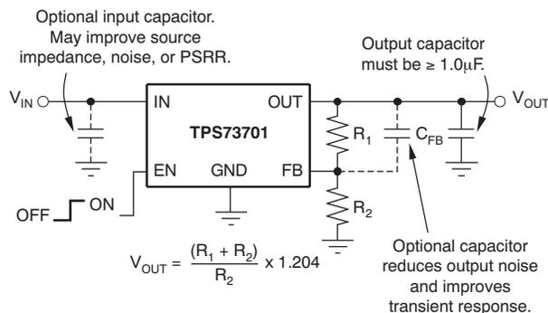
Figure 32. Typical Application Circuit for Adjustable-Voltage Version
