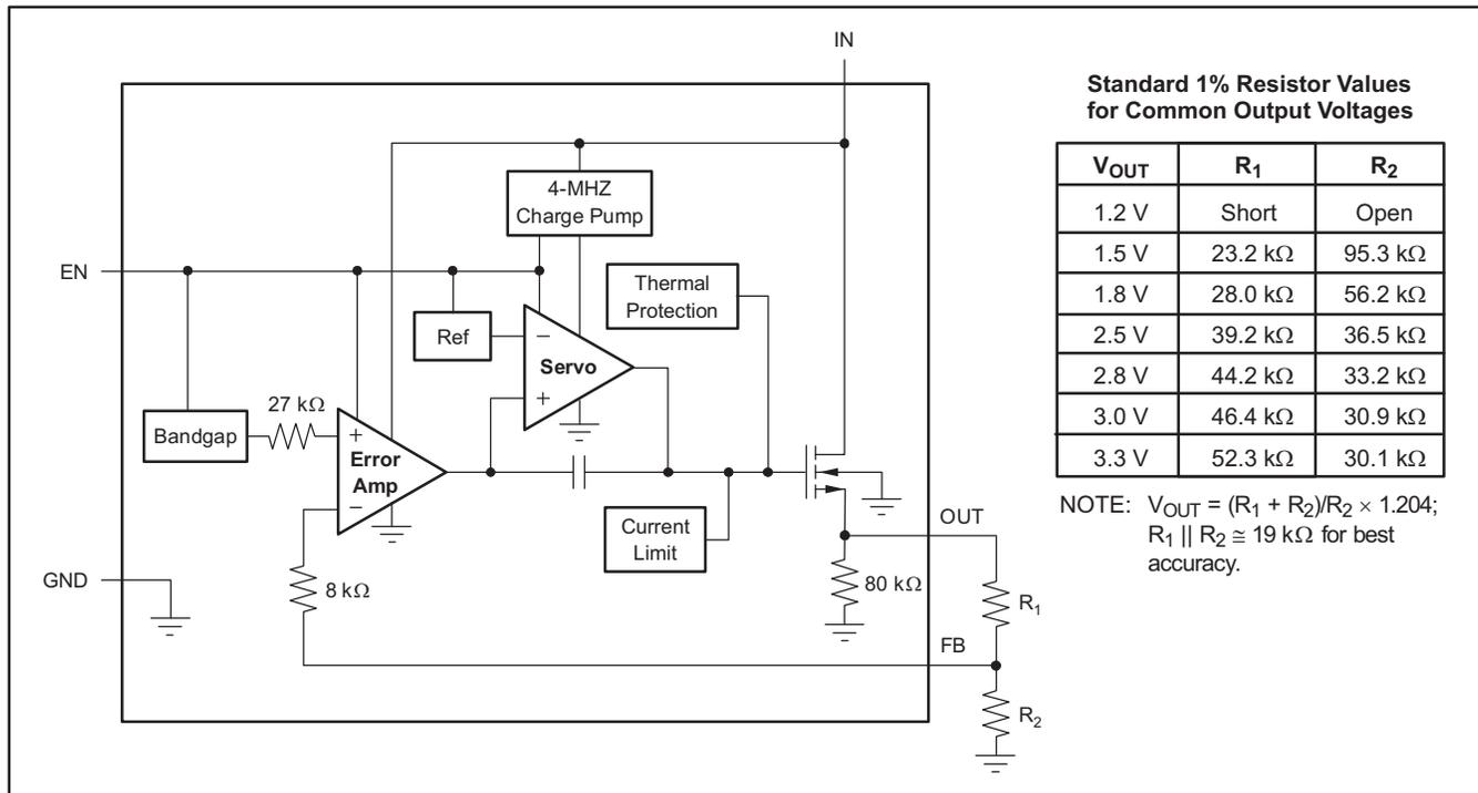
**Figure 30. Adjustable-Voltage Version**
