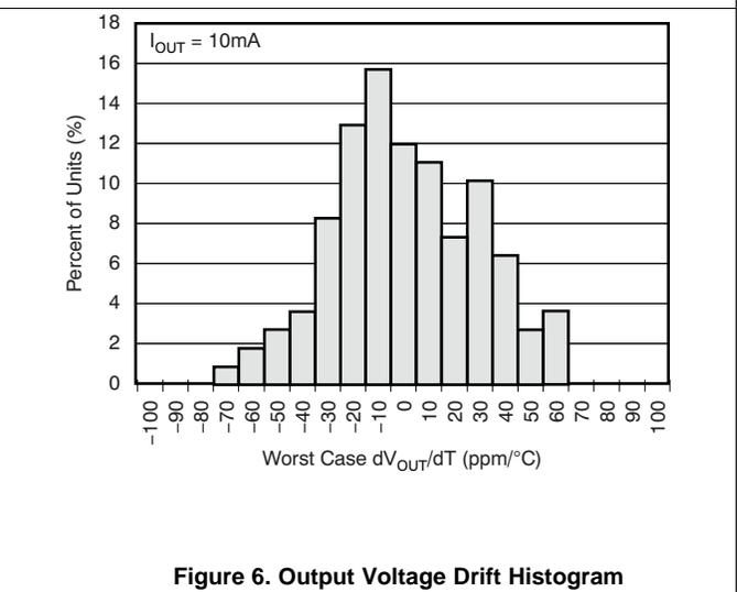
Figure 6. Output Voltage Drift Histogram
