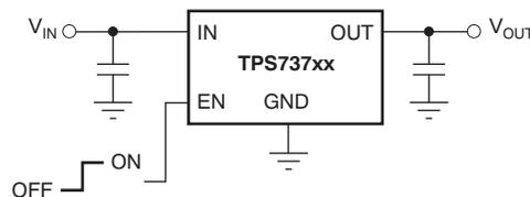
Figure 31. Typical Application Circuit for Fixed-Voltage Versions
