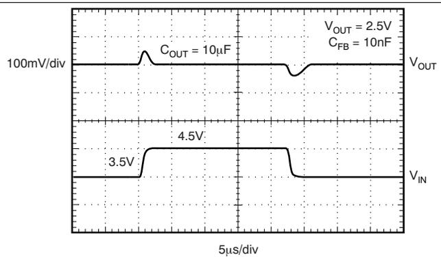
**Figure 28. TPS73701 Line Transient, Adjustable Version**
