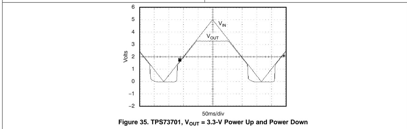
Figure 35. TPS73701,  $V_{OUT} = 3.3\text{-V}$  Power Up and Power Down
