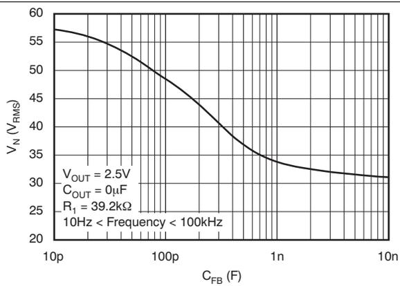
**Figure 25. TPS73701 RMS Noise Voltage vs  $C_{FB}$**
