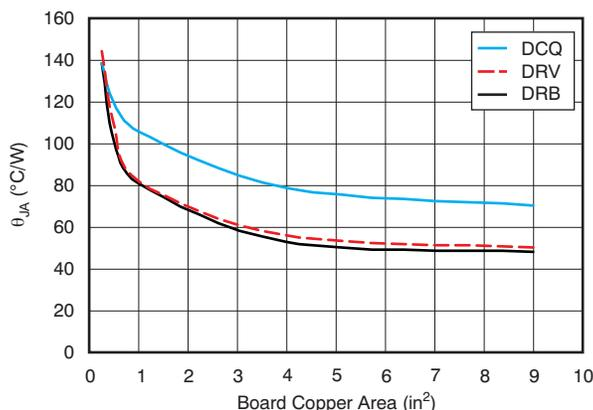
Note:  $\theta_{JA}$  value at board size of 9 in<sup>2</sup> (that is, 3 in × 3 in) is a JEDEC standard.
