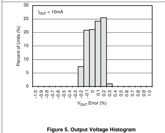
Figure 5. Output Voltage Histogram
