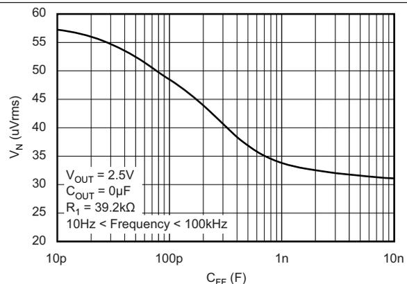
Figure 16. TPS73701 RMS Noise Voltage vs  $C_{FB}$
