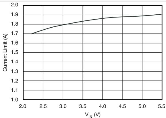
Figure 11. Current Limit vs  $V_{IN}$
