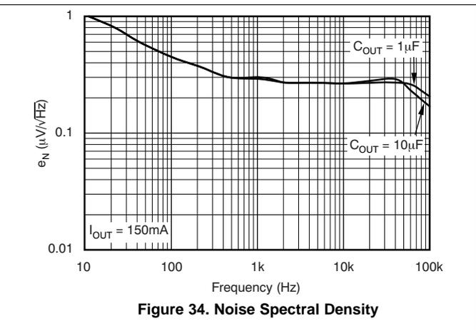
Figure 34. Noise Spectral Density
