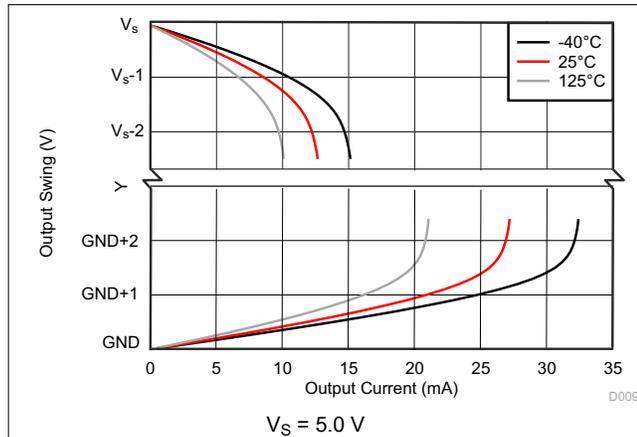
**Figure 6-5. Output Voltage Swing vs. Output Current**
