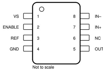
Figure 5-3. DDF Package 8-Pin SOT-23 Top View
