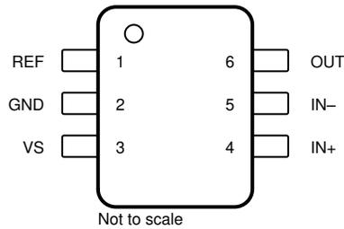
Figure 5-1. DCK Package 6-Pin SC70 Top View
