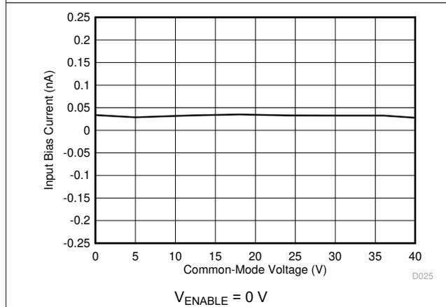
**Figure 6-7. Input Bias Current vs. Common-Mode Voltage (Shutdown)**
