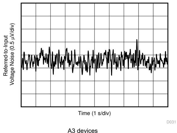
Figure 6-12. 0.1-Hz to 10-Hz Voltage Noise (Referred-To-Input)
