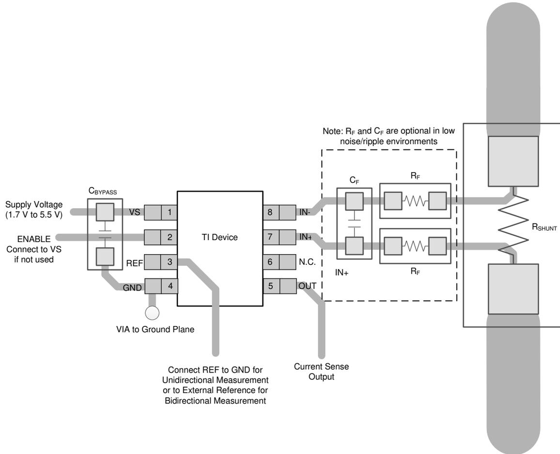
Figure 10-2. Recommended Layout for SOT-23 (DDF) Package
