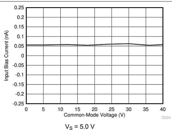
**Figure 6-6. Input Bias Current vs. Common-Mode Voltage**
