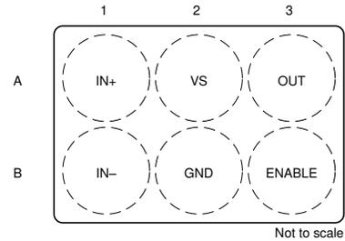
Figure 5-2. YFD Package 6-Pin DSBGA Top View
