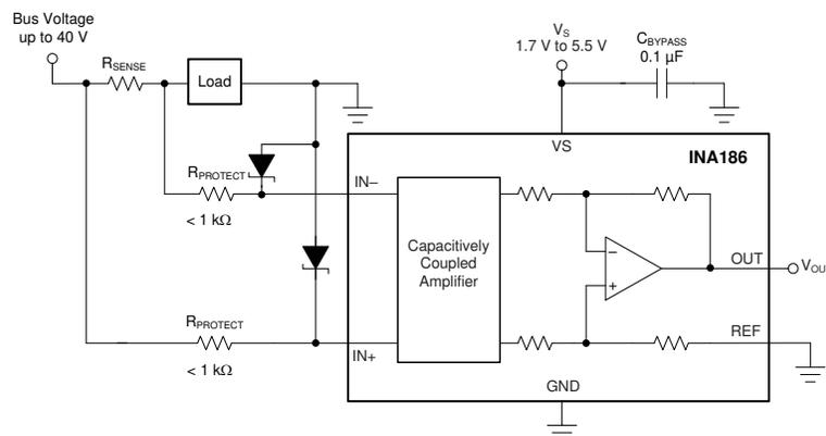
**Figure 8-4. Transient Protection Using Dual Zener Diodes**
