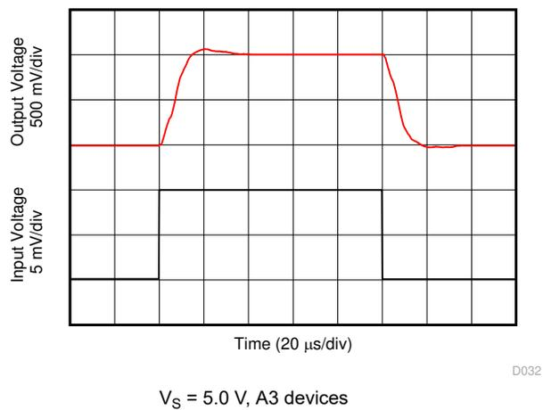
Figure 6-13. Step Response (10-mV<sub>PP</sub> Input Step)
